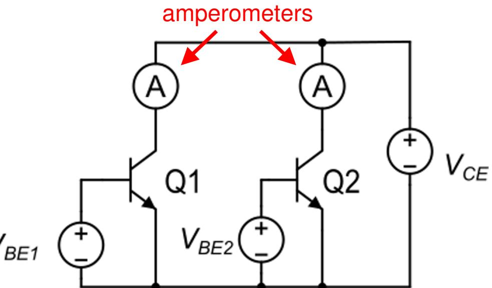
Q1 and Q2 are nominally identical and placed in the same chip. They are affected by matching errors
