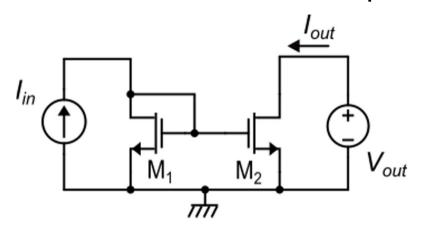
$$\begin{split} I_D &= \beta f \left( V_{GS} - V_t, V_{DS} \right) \\ I_{out} &= \beta_2 f \left( V_{GS} - V_t, V_{DS2} \right) = \beta_2 f \left( V_{GS} - V_t, V_{out} \right) \\ I_{in} &= \beta_1 f \left( V_{GS} - V_t, V_{DS1} \right) = \beta_1 f \left( V_{GS} - V_t, V_{in} \right) \\ \end{split}$$
