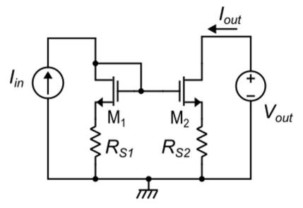
$$R_{out} = R_{S2} + r_{d2} \left( 1 + g_{m2} R_{S2} \right)$$
