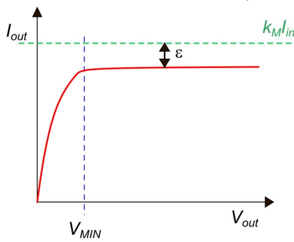
There is not an optimum voltage in the correct operating area  $(V_{out}>V_{MIN})$  at which the output currebt is equal to the ideal value
