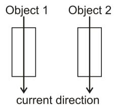
Temperature gradients develop extra voltage differences that depend on the current direction (up to several hundred µVs
