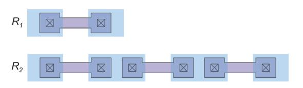
Both components R<sub>1</sub> and R<sub>2</sub> are obtained by adding different numbers of a single module.
