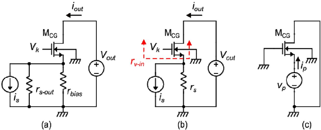
Fig. 1.1. (a) Cascode stage used as a current amplifier of unity gain; (b) fusion of the source resistance with the bias resistance (c) small signal circuit for  $r_{v\_in}$  calculation.
