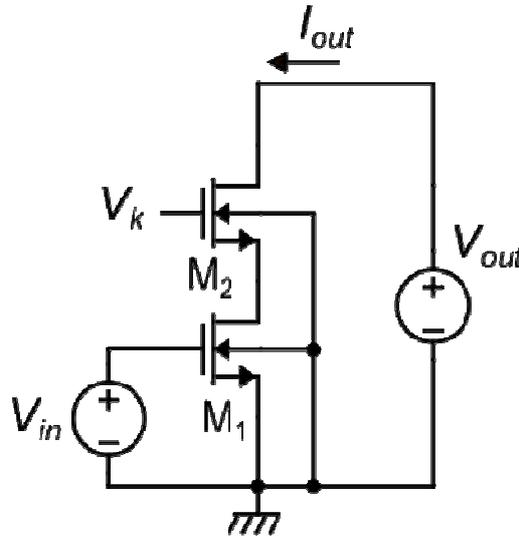
Fig. 1.2. Cascode topology with main voltages indicated.
