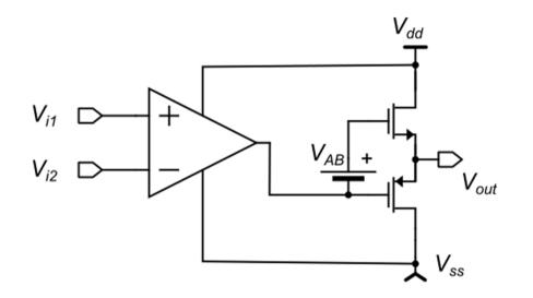
This stage looses a VGS margin to both rails. It is used only for amplifiers that can count on high supply voltage. Not used in general purposes operational amplifiers
