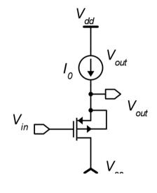
$$V_{out} = V_{in} + \left| V_{GS} \right|$$
