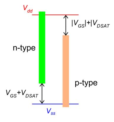
The idea is to make an n-type and ptype OTAs work together, In this way, for any value of the input common mode range, there is at least one OTA that operates correctly
