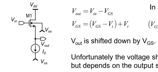
$V_{out} = V_{in} - V_{GS}$   $V_{GS} = (V_{GS} - V_t) + V_t$   $V_{GS} = \sqrt{\frac{2I_D}{\beta}}$ In strong inversion In strong inversion:
