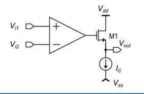
$v_{out} = A_0 v_d \frac{R_{Load}}{R_{out} + R_{Load}}$
