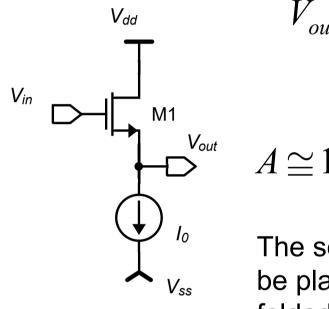
$$V_{out} = V_{in} - V_{GS}$$
