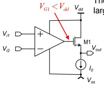
The input voltage of the source follower cannot be larger than  $V_{dd}$
