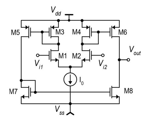
The term OTA generally indicates all single-stage amplifiers with high output resistance. The folded cascode amplifier is often classified as an OTA.
