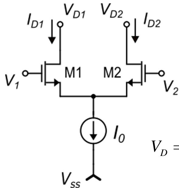
$$V_D = \sqrt{\frac{2I_{D1}}{\beta}} - \sqrt{\frac{2I_{D2}}{\beta}} = \sqrt{\frac{2}{\beta}} \cdot \left( \sqrt{I_{D1}} - \sqrt{I_{D2}} \right)$$
