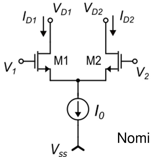
$$\begin{cases} V_1 = V_{S1} + V_{GS1} \\ V_2 = V_{S2} + V_{GS2} \end{cases} \quad V_{S1} = V_{S2} \triangleq V_S$$
