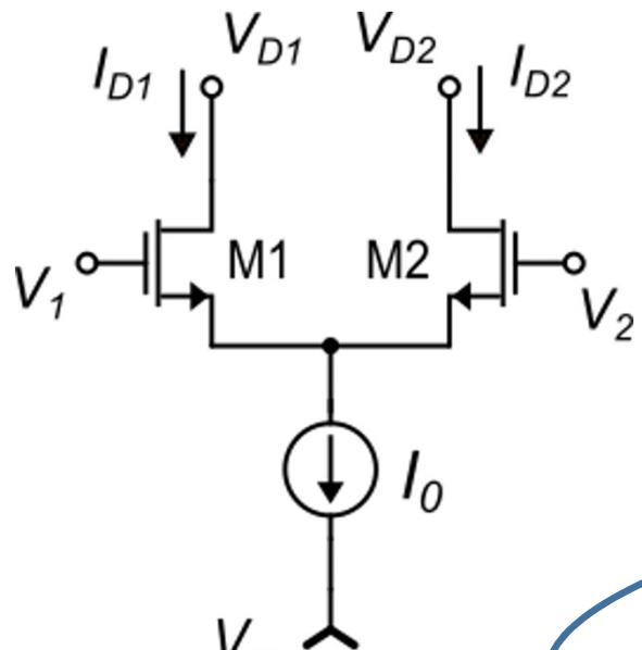
$$\left( \frac{V_D}{V_{D\text{MAX}}} \right)^2 - 1 = -2\sqrt{x(1-x)}$$
