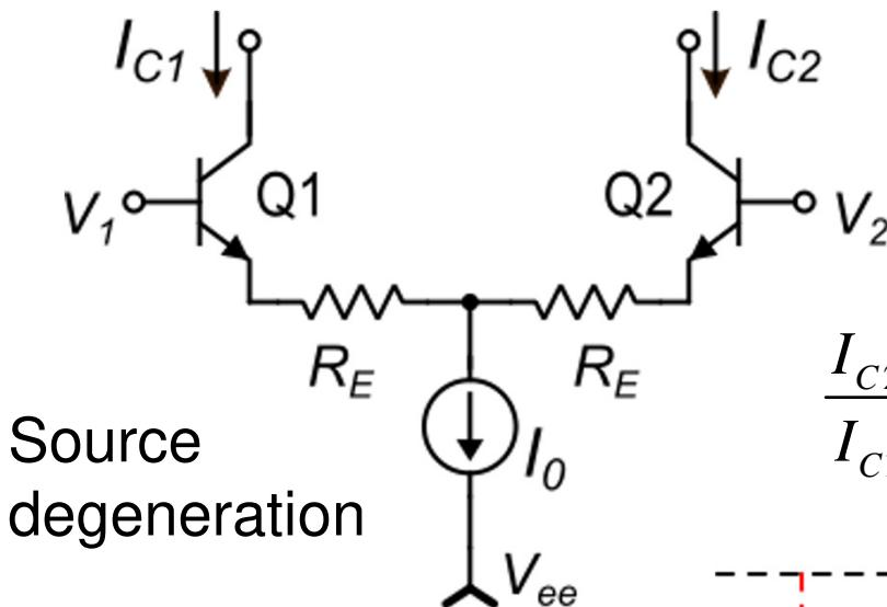
$$g_{m-rid} = \left. \frac{d(I_{C1} - I_{C2})}{dV_D} \right|_{V_D=0}$$
