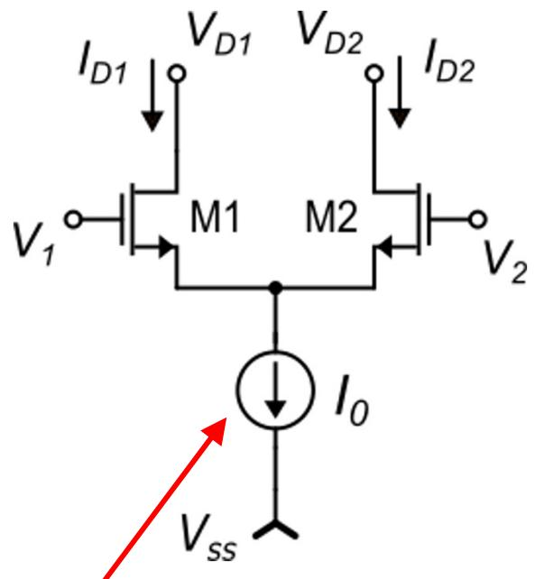
Target: obtain the relationship between the ratio  $x$  and the input differential voltage  $V_D$
