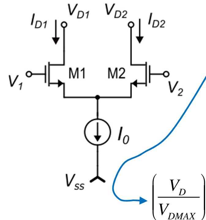
$$\frac{V_D}{V_{D\text{MAX}}} = \left[ \sqrt{x} - \sqrt{(1-x)} \right]$$
