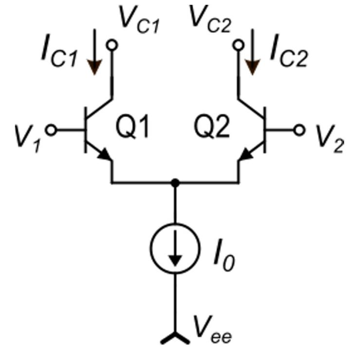
$$\left. \begin{array}{l} I_{C1} = \frac{I_0 e^{\frac{-V_D}{V_T}}}{1 + e^{\frac{-V_D}{V_T}}} \\ I_{C2} = \frac{I_0 e^{\frac{-V_D}{V_T}}}{1 + e^{\frac{-V_D}{V_T}}} \end{array} \right\}$$
