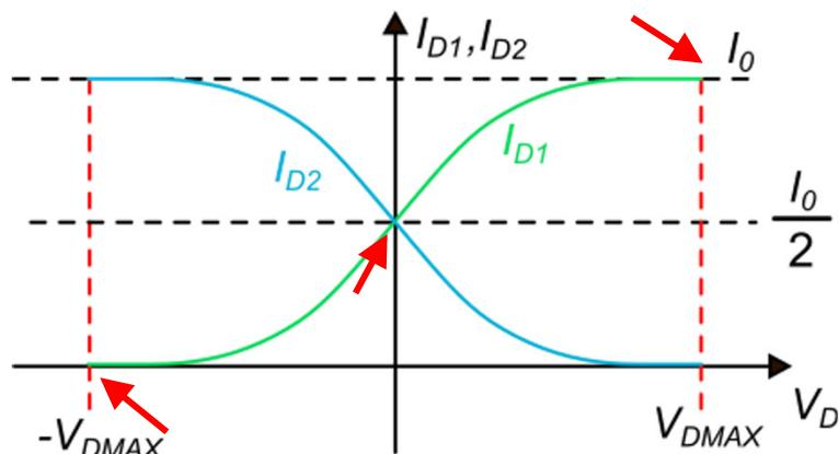
$$\left\{ \begin{array}{l} V_D = \pm V_{D\text{MAX}} \rightarrow \frac{dI_{D1}}{dV_D} = 0 \quad \sqrt{\frac{2I_0}{\beta}} \triangleq V_{D\text{MAX}} \\ V_D = 0 \rightarrow \frac{dI_{D1}}{dV_D} = \frac{I_0}{\sqrt{2}V_{D\text{MAX}}} = \sqrt{\frac{I_0^2 \beta}{4I_0}} = \frac{1}{2} \sqrt{\beta I_0} \end{array} \right.$$
