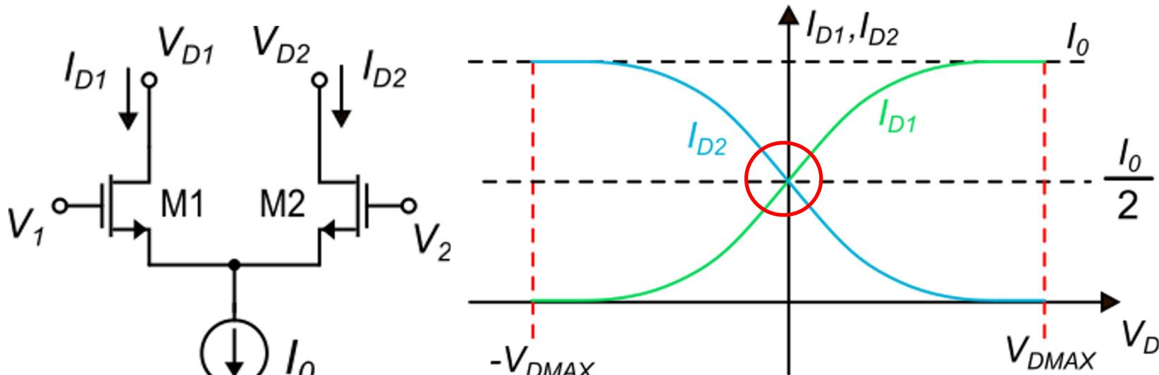
$$\left\{ \begin{array}{l} I_{D1} \approx \frac{I_0}{2} + v_d \left. \frac{dI_{D1}}{dV_D} \right|_{V_D=0} = \frac{I_0}{2} + \frac{g_m}{2} v_d \\ I_{D2} \approx \frac{I_0}{2} + v_d \left. \frac{dI_{D2}}{dV_D} \right|_{V_D=0} = \frac{I_0}{2} - \frac{g_m}{2} v_d \end{array} \right.$$
