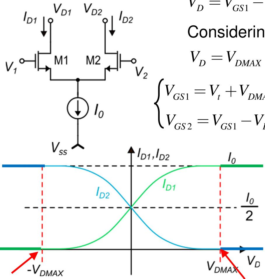
$$V_D = V_{GS1} - V_{GS2} \Rightarrow V_{GS2} = V_{GS1} - V_D$$
