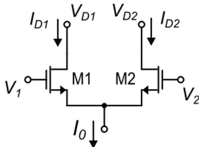
**Inputs:**  $V_1, V_2$  (effective input signal:  $V_D = V_1 - V_2$ )
