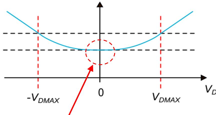
For small differential voltages ( $v_d \ll V_{DMAX}$ ), the source potential is practically constant.
