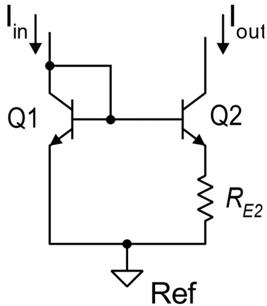
$$\Delta V_{BE} \triangleq V_{BE1} - V_{BE2} = R_{E2} I_{E2} \cong R_{E2} I_{C2}$$
