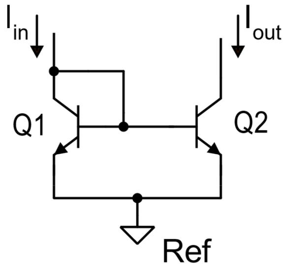
$$V_{IN} = V_{CE1} = V_{BE1} \approx V_\gamma$$
