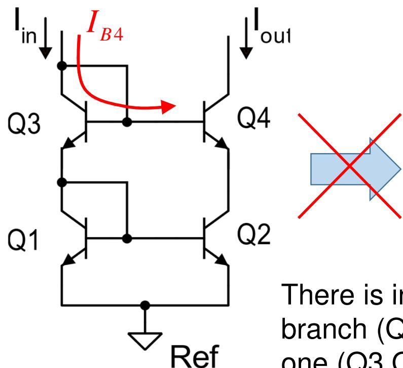
There is interaction of the output branch (Q2,Q4) with the input one (Q3,Q4) caused by the base currents. This interaction is not present in the cascode MOSFET
