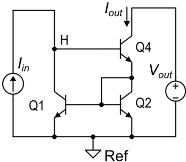
In the Wilson current mirror the relative error due to the base current is of the order of  $1/\beta^2$  only when it is designed for  $k_M=1$ . For current gains different from one, the relative error becomes of the order of  $1/\beta$ .
