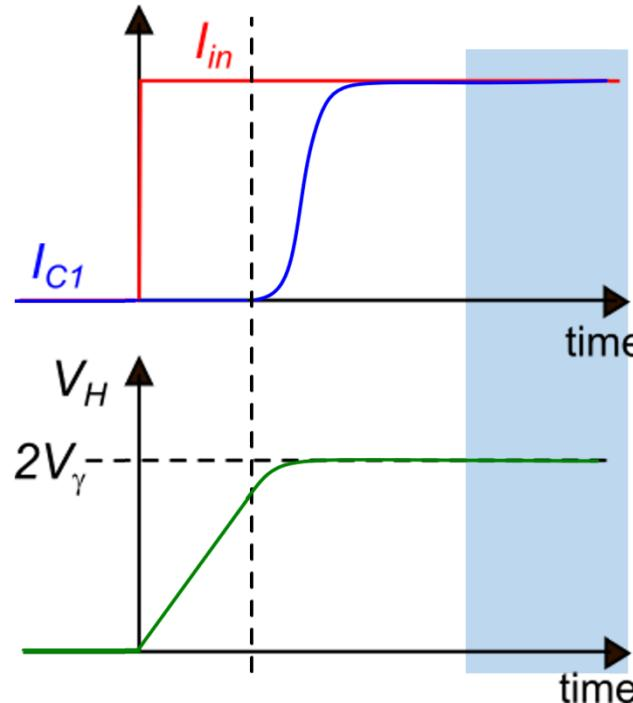
Due to the exponential law, small  $V_H$  increments produce large  $I_{C2}$  (and then  $I_{C1}$ ) increases
