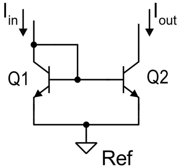
$$\frac{I_{C2}}{I_{C1}} = k_M \quad \frac{I_{out}}{I_{in}} = k_M \frac{1}{1 + \frac{1 + k_M}{\beta}} < k_M$$
