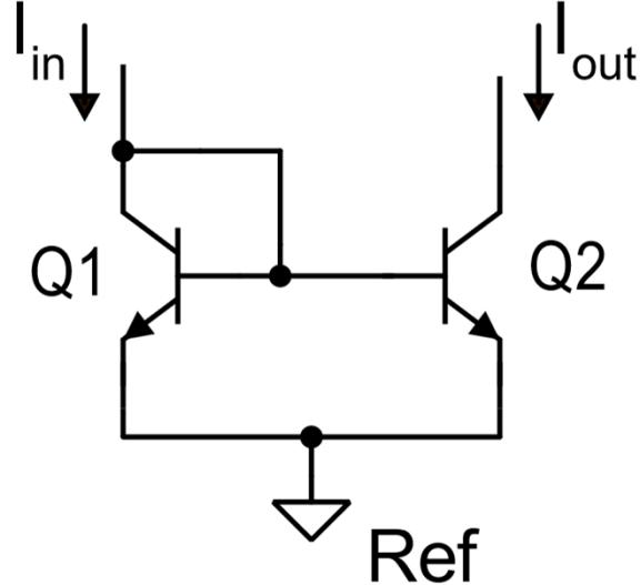
$$I_{C2} = I_{S2} e^{\frac{V_{BE}}{V_T}} \left( 1 + \frac{V_{CB2}}{V_A} \right) = I_{S2} e^{\frac{V_{BE}}{V_T}} \left( 1 + \frac{V_{CE2}}{V_A} - \frac{V_{BE}}{V_A} \right)$$
