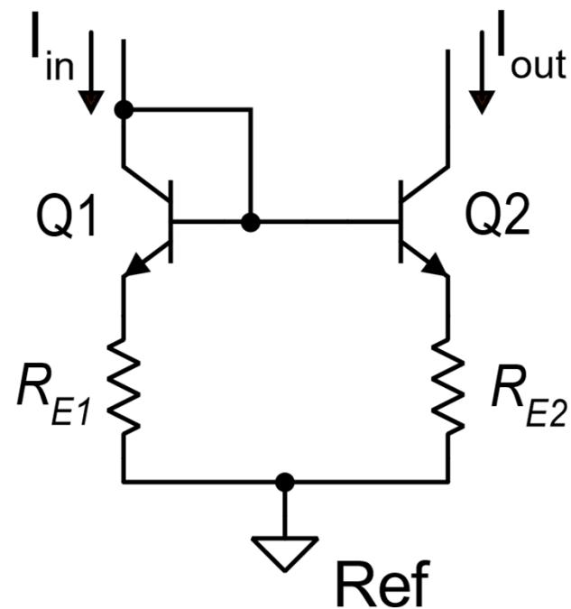
$$k_M = \frac{I_{S2}}{I_{S1}} = \frac{A_{E2}}{A_{E1}} = \frac{\text{area}_2}{\text{area}_1} = \frac{I_{C2}}{I_{C1}}$$
