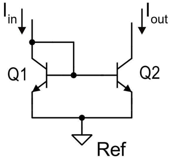
$$\frac{I_{C2}}{I_{C1}} = k_M \quad I_{C2} = I_{out}$$
