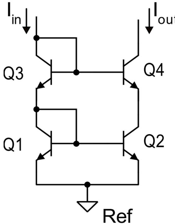
$$\left\{ \begin{array}{l} I_{out} = I_{C4} = I_{E4} - I_{B4} = I_{C2} - I_{B4} \\ I_{in} = I_{C1} + I_{B1} + I_{B2} + I_{B4} \end{array} \right.$$
