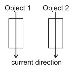
Temperature gradients develop extra voltage differences that depend on the current direction (up to several hundred µVs
