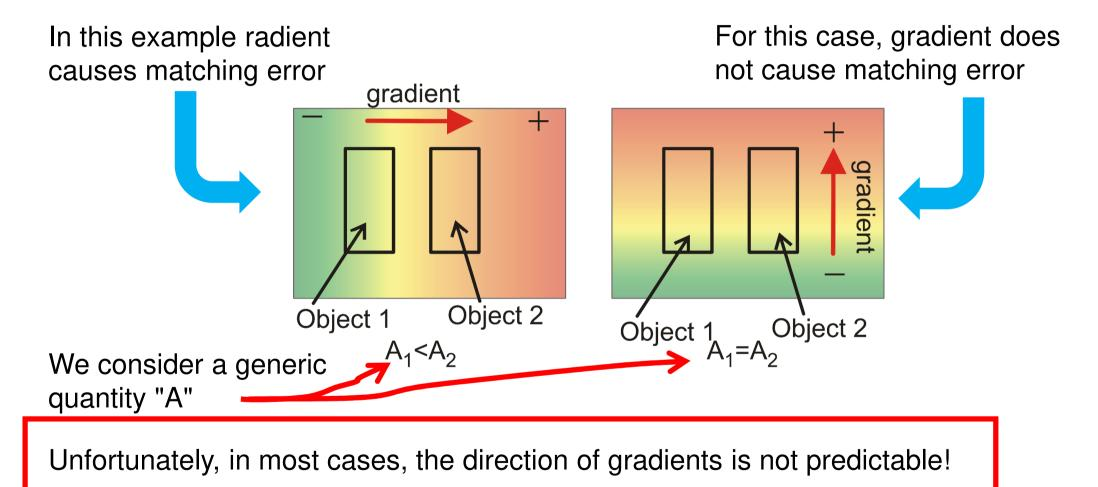
Layout rules that prevent device mismatch caused by gradients
