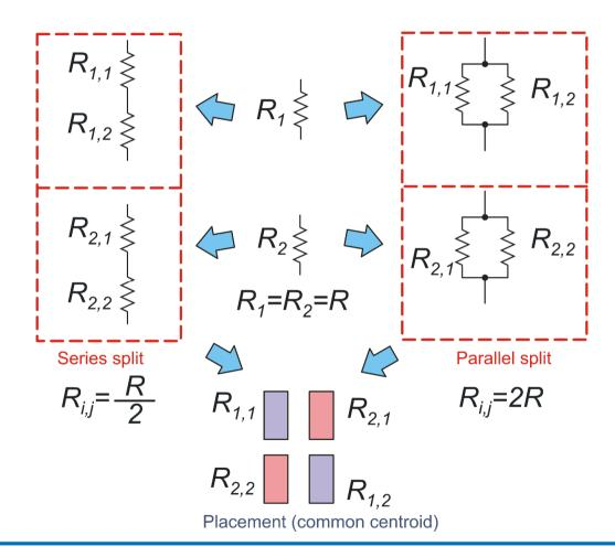
Split and connect components in common centroid configurations
