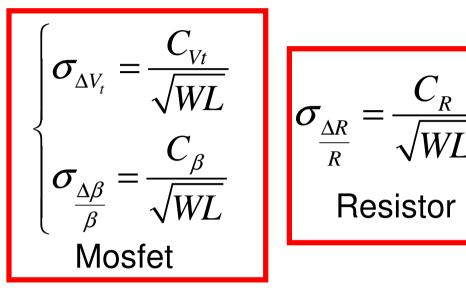
$C_{vt}$ ,  $C_{\beta}$  and  $C_{R}$  are constant parameters of the process Their values are given in the Design Rule Manual, with names that depend on the foundry (there is no general convention).  $C_{vt}$  units are generally V·µm, while  $C_{\beta}$  and  $C_{R}$  ones are µm.
