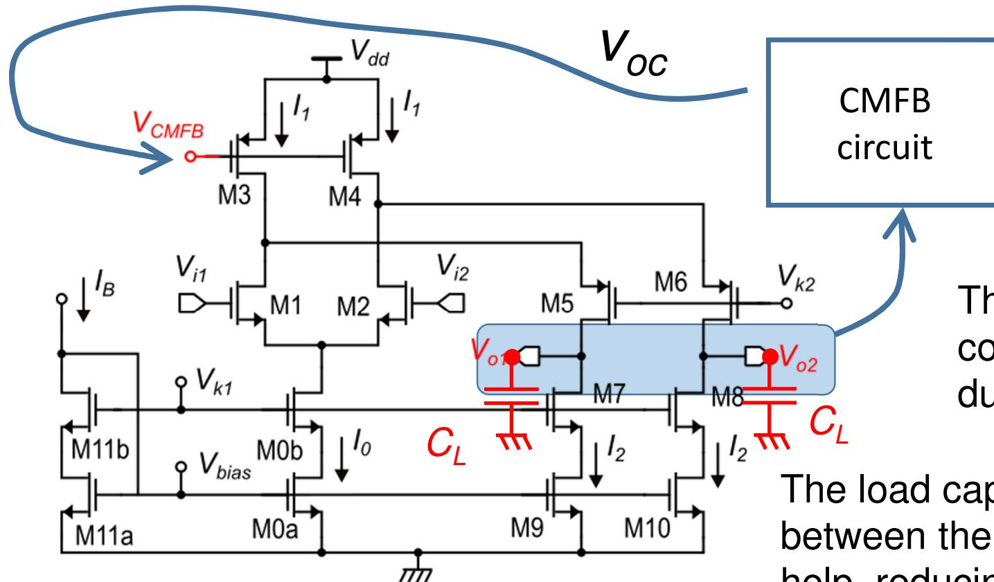
Considering small signal components, this is a feedback loop that can lead to instability
