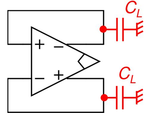
Unity gain case with only load capacitance to gnd
