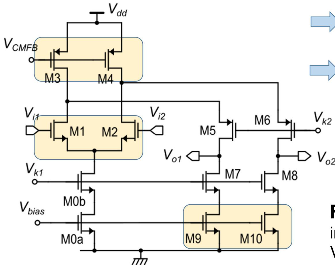
$$\begin{aligned} F_3 &= \frac{g_{m3}}{g_{m1}} = \frac{I_{D3}}{I_{D1}} \frac{V_{TE1}}{V_{TE3}} = 2 \frac{V_{TE1}}{V_{TE3}} \\ F_9 &= \frac{g_{m9}}{g_{m1}} = \frac{I_{D9}}{I_{D1}} \frac{V_{TE1}}{V_{TE9}} = \frac{V_{TE1}}{V_{TE9}} \end{aligned}$$
