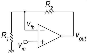
Just after a step variation of the input voltage, the feedback voltage, derived by the output voltage, cannot change instantaneously and the input differential voltage of the opamp can be driven out of the linearity region of the first stage
