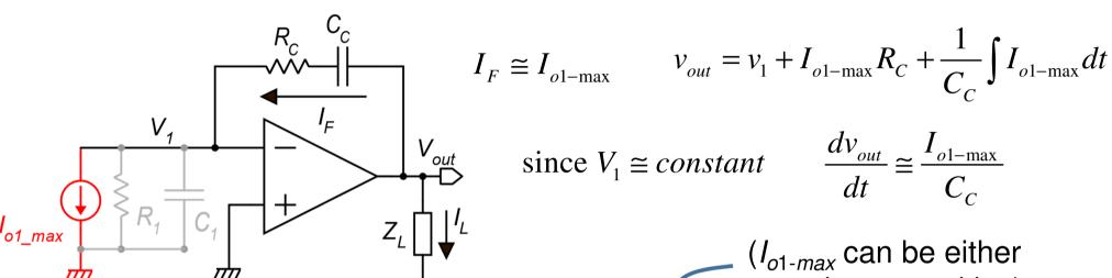
If the gain of the second stage is high enough, we can consider virtual gnd at input  $v_1$ .
