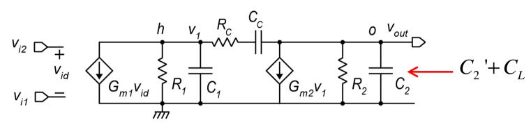
We have designed the op-amp for the maximum  $C_L$ . It must be stable also for smaller values
