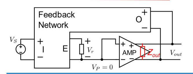
$$\frac{v_{out}}{v_{s}} = -\frac{\alpha}{\beta} + \gamma$$
