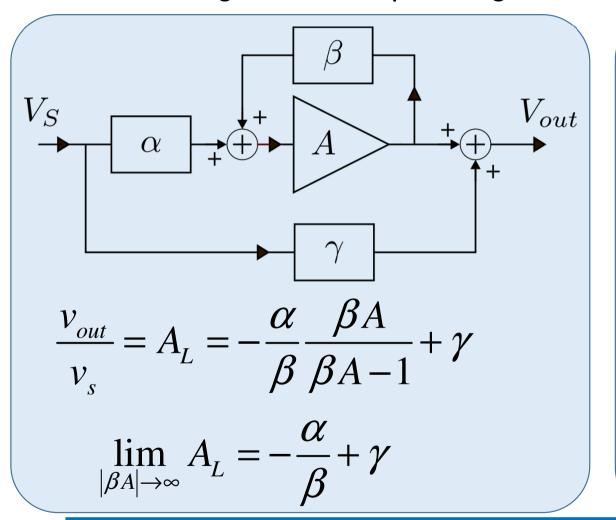
$$\frac{v_{out}}{v_s} = A_L = -\frac{\alpha}{\beta} \frac{\beta A}{\beta A - 1}$$
