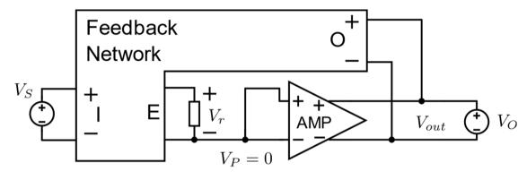
$$\frac{v_{out}}{v_s} = \frac{\alpha^*}{\beta} \frac{\beta A}{\beta A - 1} + \frac{\gamma}{1 - \beta A}$$
