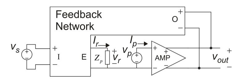
$$Z_{i} = \left(\frac{v_{p}}{i_{p}}\right)_{v_{s}=0}; \quad \beta \equiv \left(\frac{v_{r}}{v_{out}}\right)_{v_{s}=0}; \quad A = \left(\frac{v_{out}}{v_{p}}\right)_{v_{s}=0} \qquad \frac{1}{Z_{p}} = \frac{1}{Z_{i}} + \frac{\rho}{\alpha}(1-\beta A)$$
