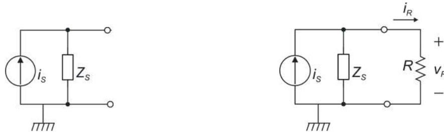
Fig. 1.7. Norton equivalent circuit of a source whose output of interest is a current (left); Direct connection of the sensor to a resistance, in order to operate current-to-voltage conversion.
