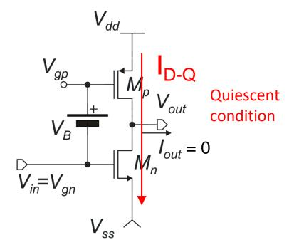
$$I_{DN-Q} = \frac{\beta_n}{2} \left( V_{GSn-Q} - V_{tn} \right)^2$$
