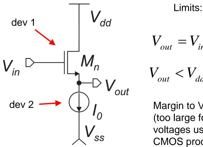
$$V_{out} = V_{in} - V_{GS}$$
