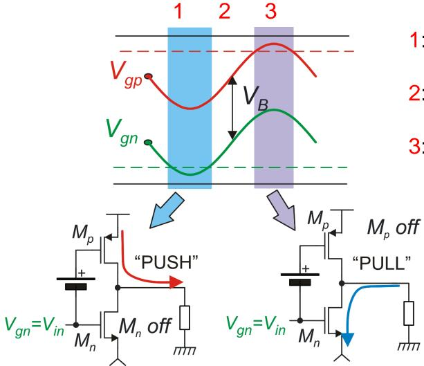
1: M<sub>n</sub> off, M<sub>p</sub> on
