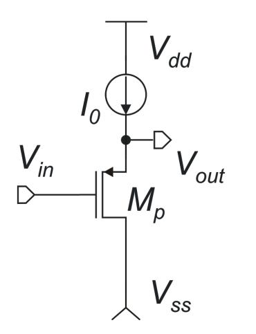
$$V_{out} = V_{in} + \left| V_{GS} \right|$$
