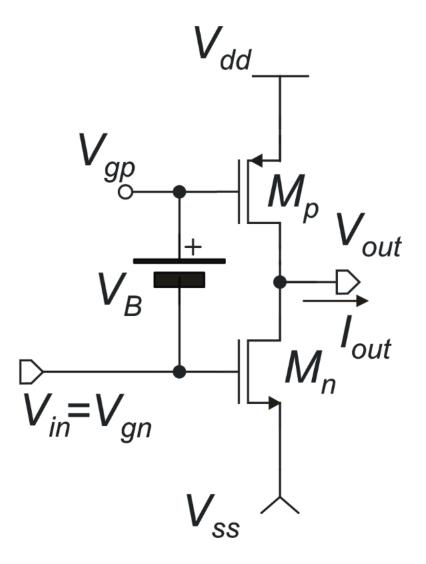
The difference from the class-A common source output stage is the fact that also Mp is driven by the input signal. This is obtained by driving the gate of Mp with a shifted version of the input signal. The voltage shifter is represented by battery  $V_B$ . For obvious reasons, a real battery is not used and a voltage shifter is used. There are several different way to implement the voltage shifter to be used to replace the battery  $V_B$ .
