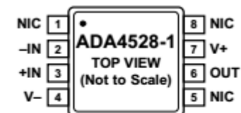
Figure 1. ADA4528-1 Pin Configuration, 8-Lead MSOP
