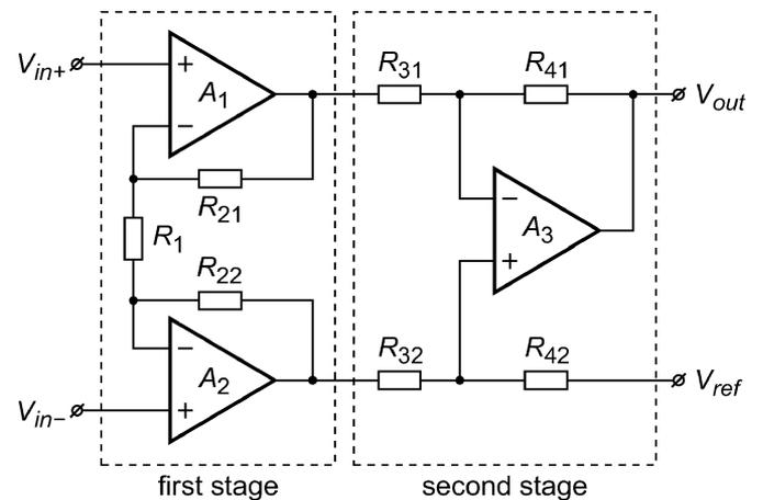
Fig. 3. Conventional 3-opamp instrumentation amplifier.
