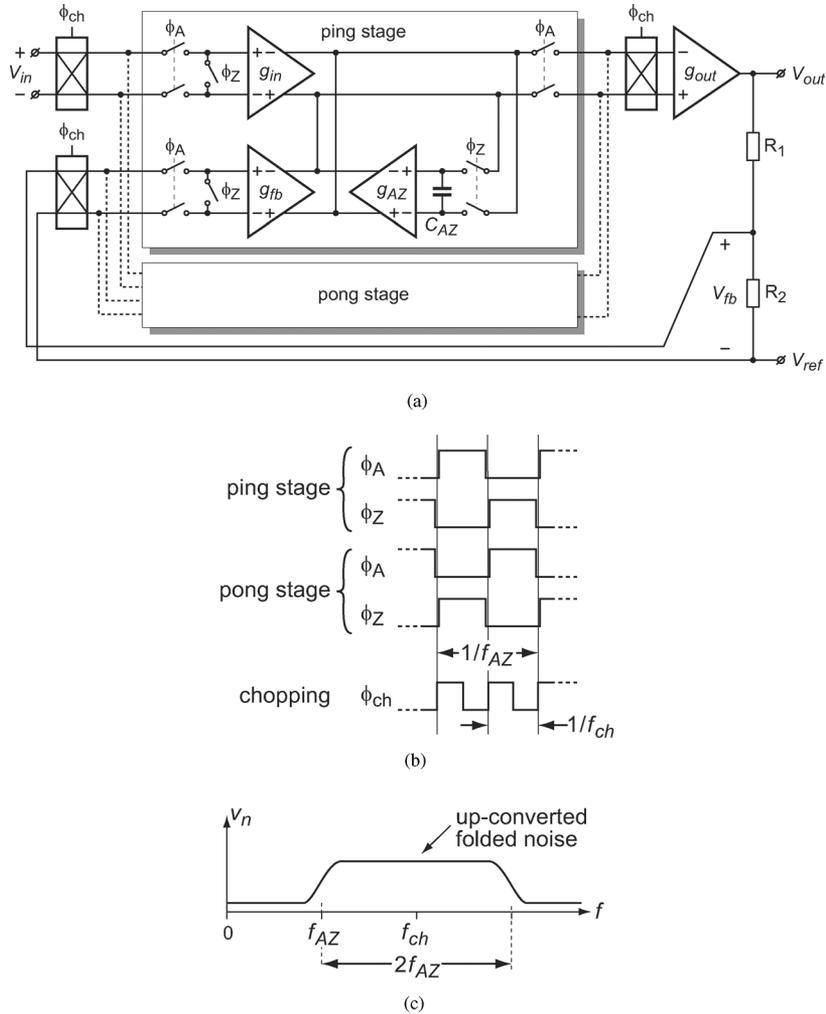
Fig. 9. A ping-pong auto-zeroed CFIA chopped at  $f_{ch} = 2f_{AZ}$ : (a) block diagram, (b) timing diagram, (c) input-referred noise PSD.
