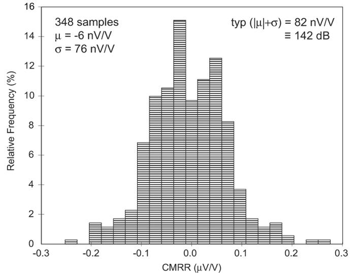
Fig. 20. Histogram of the amplifier's CMRR in a CMVR from 0.1 V below the negative supply to midsupply, measured with a gain of 1000x at a supply of 5 V.
