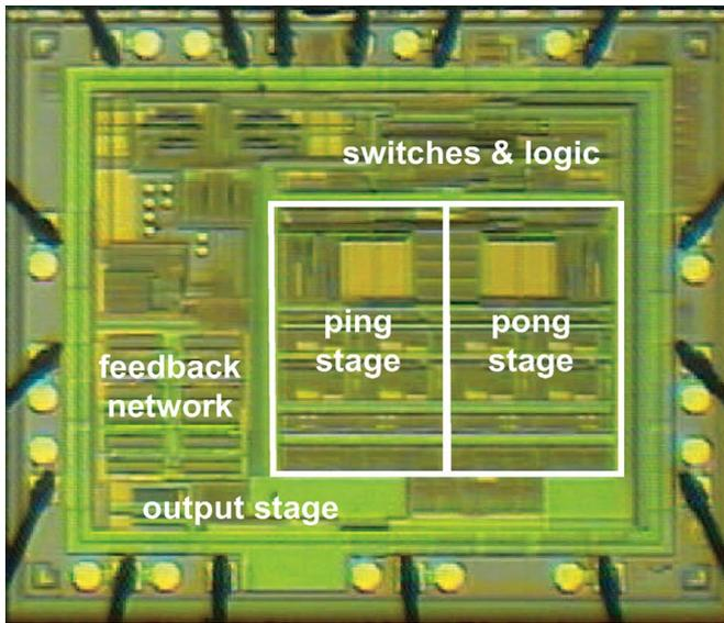
Fig. 18. Chip microphotograph of the instrumentation amplifier.
