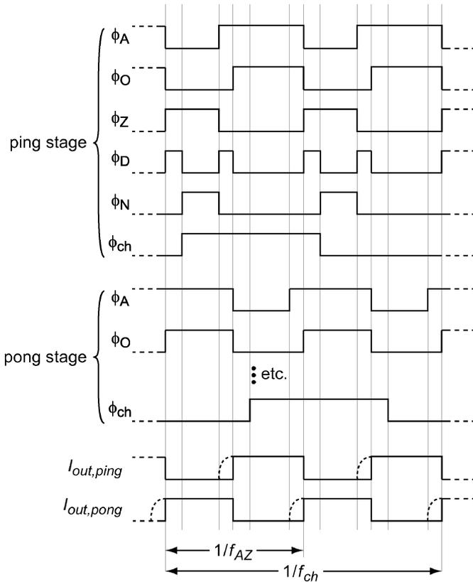
Fig. 15. Timing diagram of the ping-pong stages.
