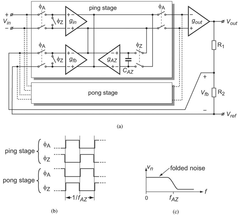
Fig. 7. A ping-pong auto-zeroed CFIA: (a) block diagram, (b) timing diagram, (c) input-referred noise PSD.
