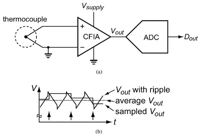
Fig. 1. (a) Current-feedback instrumentation amplifier interfacing between a grounded sensor and an ADC. (b) Error due to sampling of output ripple by the ADC.
