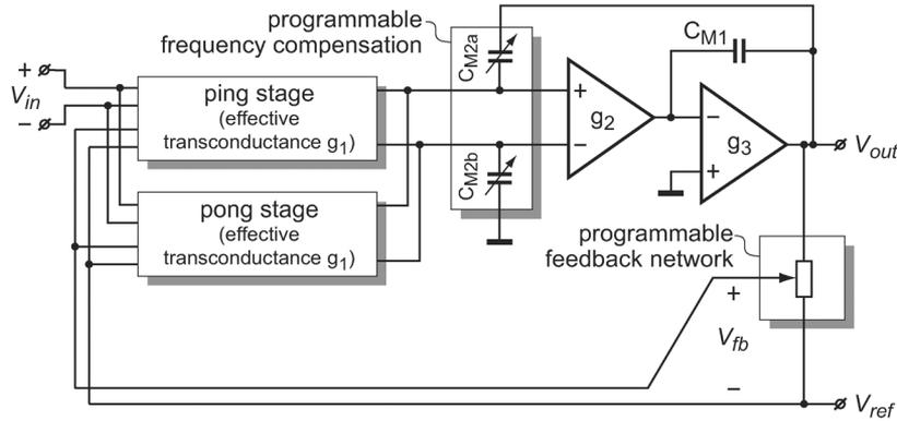
Fig. 13. Simplified circuit diagram of the instrumentation amplifier.
