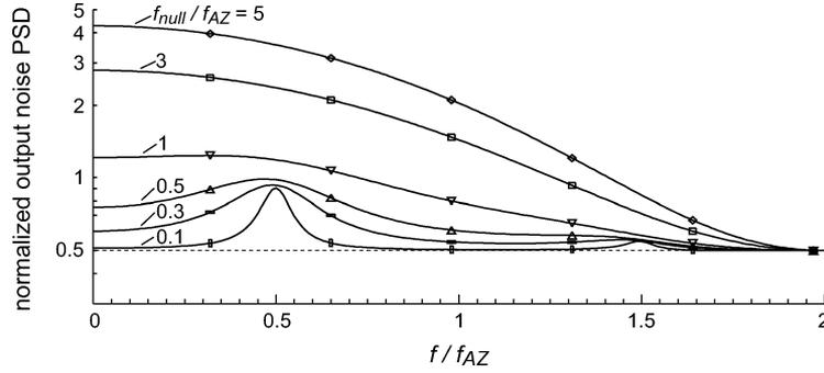
Fig. 12. Simulated noise PSD of an auto-zeroed amplifier chopped  $f_{ch} = f_{AZ}/2$  for different values of  $f_{null}$ .
