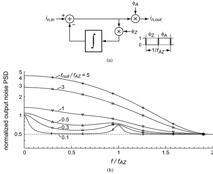
Fig. 11. Auto-zeroing with a slow-settling nulling loop: (a) model of the nulling loop, in which the bandwidth  $f_{null}$  is set by unity-gain frequency of the integrator; (b) simulated output noise PSD for different values of  $f_{null}$ , normalized to the input noise PSD.
