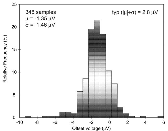
Fig. 21. Histogram of the amplifier's input-referred offset voltage measured with a gain of 1000x at a supply of 5 V.
