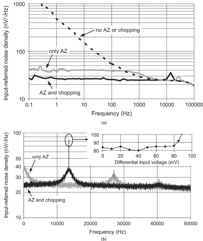
Fig. 19. Measured input-referred noise spectra: (a) on a logarithmic frequency scale; (b) on a linear frequency scale, with inset showing the PSD at the chopping frequency as a function of the differential input voltage. Measurements were performed with a resolution bandwidth of 10 Hz.
