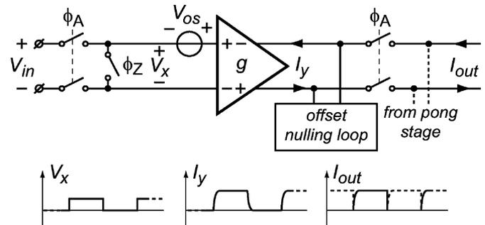
Fig. 8. Switching transients in an auto-zeroed transconductor.
