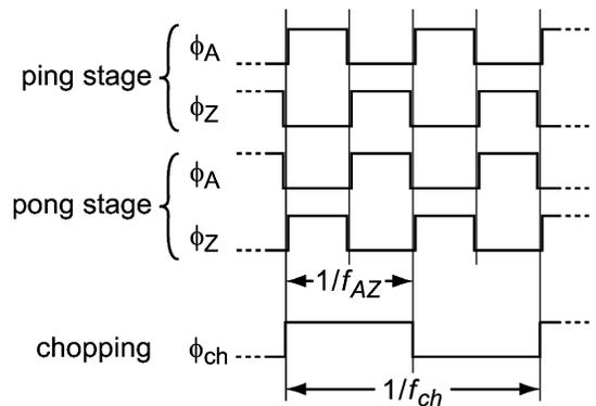
Fig. 10. Timing diagram of a ping-pong auto-zeroed CFIA chopped at  $f_{ch} = f_{AZ}/2$ .
