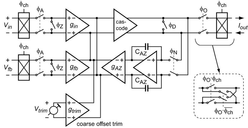
Fig. 14. Circuit diagram of the ping-pong stages.
