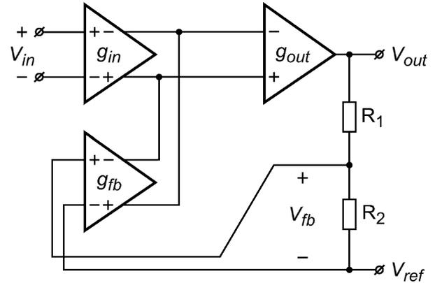
Fig. 2. A typical current-feedback instrumentation amplifier.
