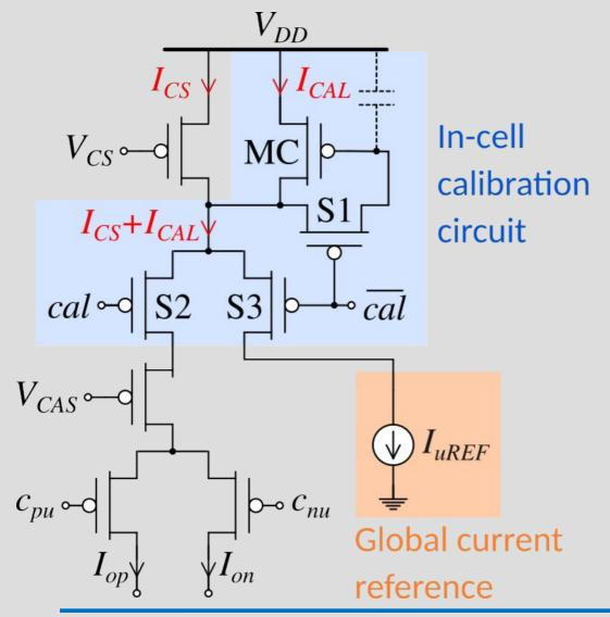
More switches (S1-S3) are added to the stack + a periodic calibration phase (*cal*) for each cell
