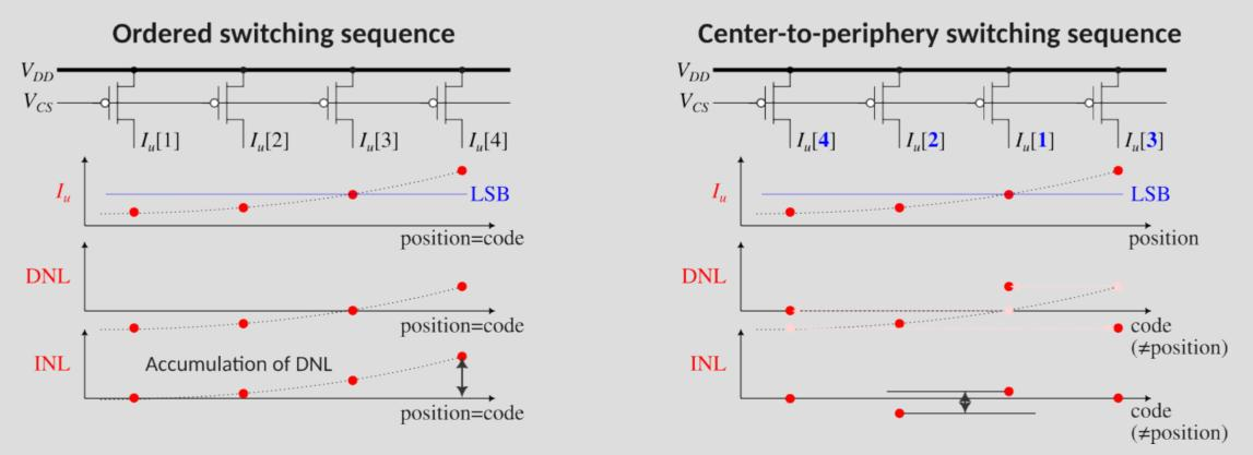
If we activate the CS in an orderly fashion: the gradient errors will accumulate  $\rightarrow$  large INL If the activation sequence starts from the center devices and hops to the outer ones, DNL is almost the same (statistically), but INL error gets tighter Resembles the **common centroid** layout technique
