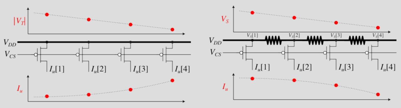
Nominally identical devices, under same bias conditions gives different currents due to: Manufacturing imperfections (e.g. threshold parameter spreading) Interconnection ohmic drops Both results in current gradients The switching order is decided by the digital logic Both results in current gradients The switching order is decided by the digital logic
