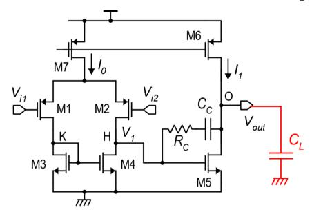
Hypotheses 1 and 2 correspond to consider that all parasitic capacitances of the amplifier are negligible with respect to  $C_i$  and  $C_{C}$ , which are external to the amplifier  $(C_i)$  or are purposely placed devices  $(C_C)$ .
