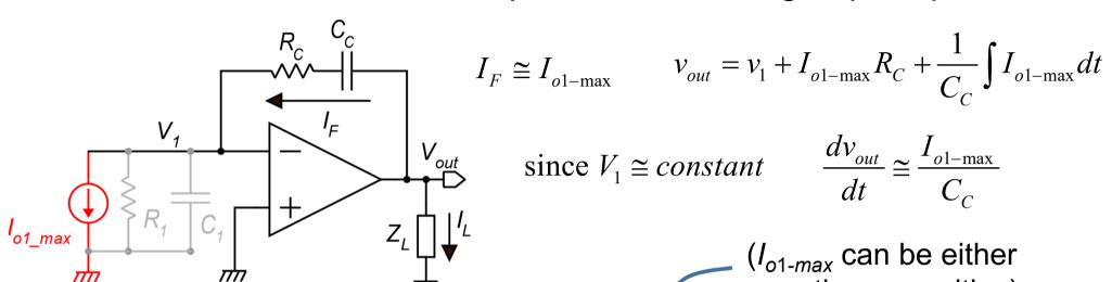
If the gain of the second stage is high enough, we can consider virtual gnd at input v₁.
