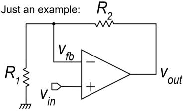
Just after a step variation of the input voltage, the feedback voltage, derived by the output voltage, cannot change instantaneously and the input differential voltage of the opamp can be driven out of the linearity region of the first stage
