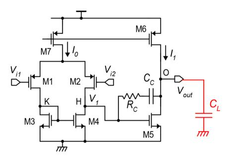
$$GBW \cong \underbrace{\frac{1}{2\pi\sigma}}_{C_{GS5}} \underbrace{\frac{g_{m5}}{C_{GS5}}}_{C_{GS5}} \underbrace{\frac{1}{1 + \frac{C_L}{C_{GS5}}}}_{C_{GS5}}$$
