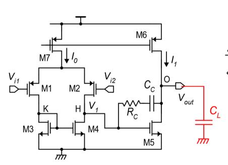
$$I_{supply} = 2\pi\sigma \cdot GBW \cdot C_L \cdot \left(V_{TE5} + 2\frac{g_{m1}}{g_{m5}}V_{TE1}\right)$$
