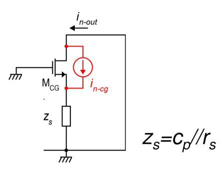
Every time we have a floating current source, we can split it into two sources with one terminal at ground
