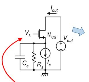
Hypothesis:  $V_k$  is at gnd in the small signal circuit. For example, it is provided by an ideal voltage source
