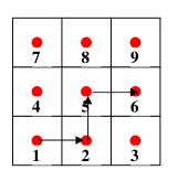
*arcs* join the point  $P_r$  to point  $P_s$  if  $a_{rs} \neq 0$ . A graph is strictly connected if for any couple  $P_i$  and  $P_j$  of points there exists an oriented path leading from  $P_i$  to  $P_j$ .
