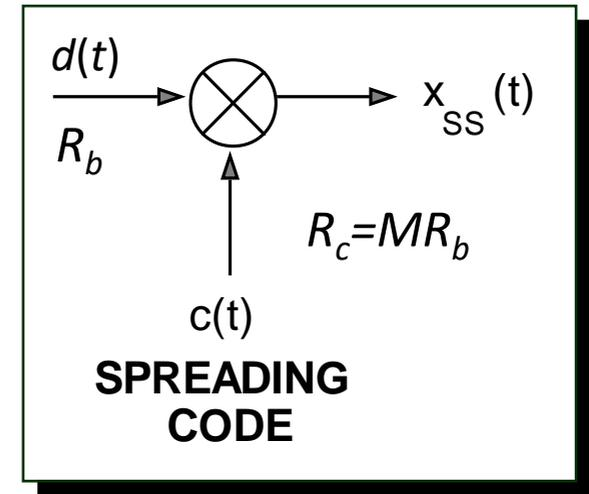
*We can add a data message on top of the ranging code and create a proper DS/SS signal*
