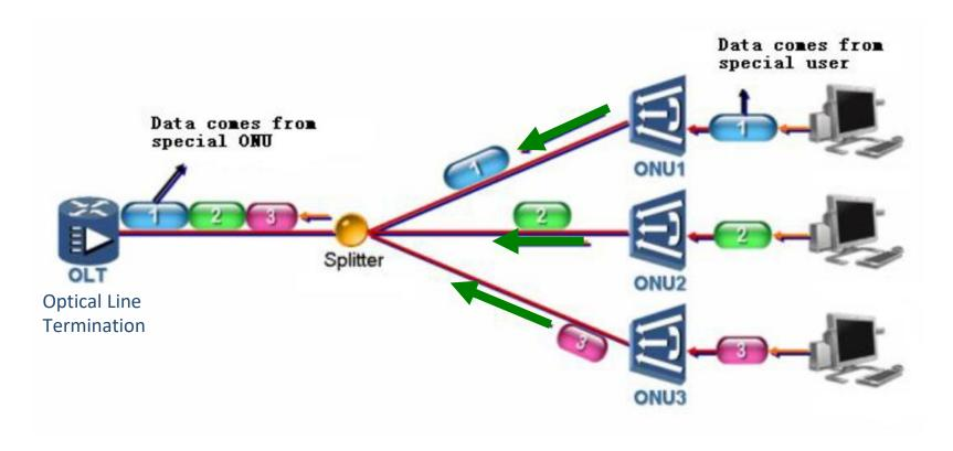
In a GPON Network, upstream and downstream data packets are transmitted in wavelengths in the 1290-1330nm (typ. 1310) and 1480-1500nm (typ. 1490) ranges respectively.
