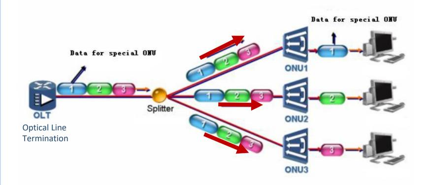
In a GPON Network, upstream and downstream data packets are transmitted in wavelengths in the 1290-1330nm (typ. 1310) and 1480-1500nm (typ. 1490) ranges respectively.
