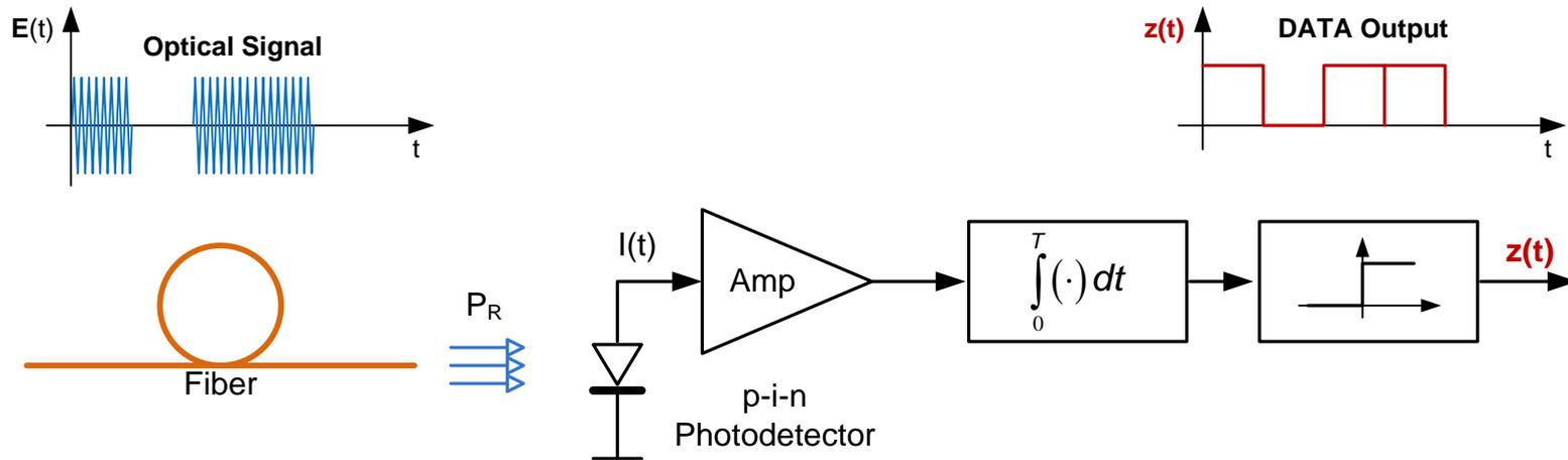
**Key Components: LASER and Photodetector (photodiode)**
