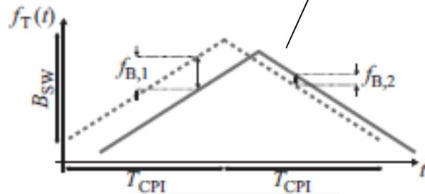
$$f_{B,1} = f_D + f_\tau = -\frac{2}{\lambda} v_r - \frac{2B_{sw}}{cT_{CPI}} R$$
