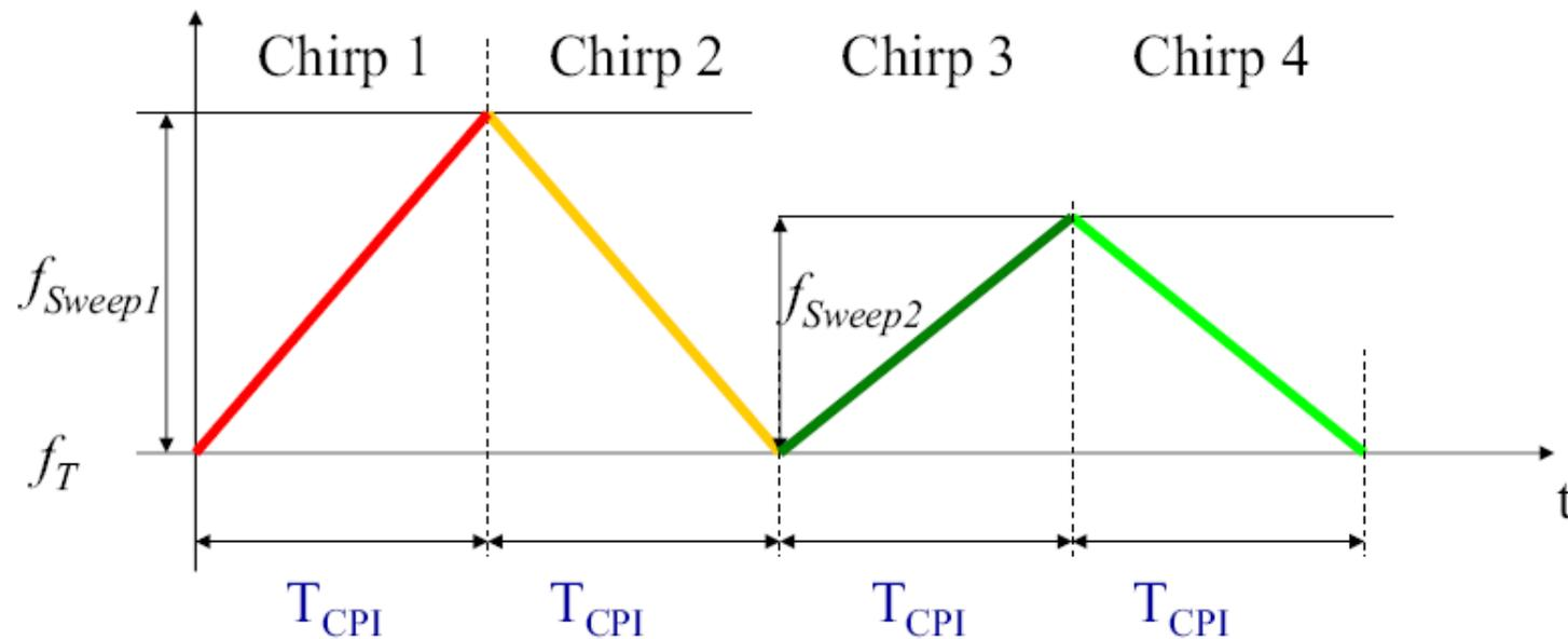
With only one up and down chirp, two targets are ambiguous. With four chirps two targets can be easily resolved
