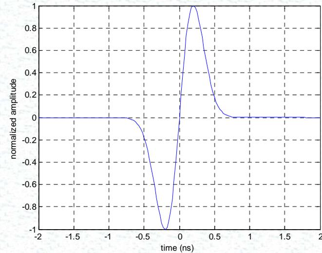
Waveform of UWB SRR, Gaussian pulse
