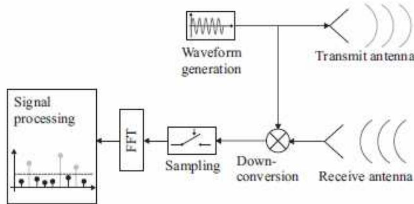
FFT: applied on each segment (up and down chirp)
