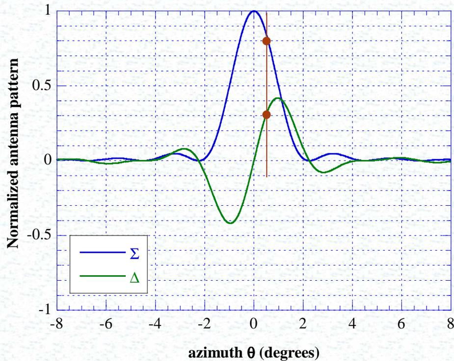
Example, with Gaussian antenna pattern and -3dB beamwidth=3°
