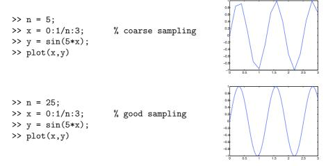
The solid line is used by plot by default. It is possible to change the style and the color, e.g.:
