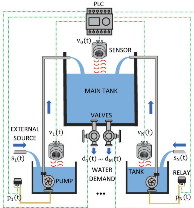
Fig. 1. Illustration of a reference scenario of water distribution
