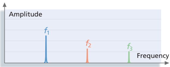
Corresponding frequency spectrum obtained by a Fourier transform
