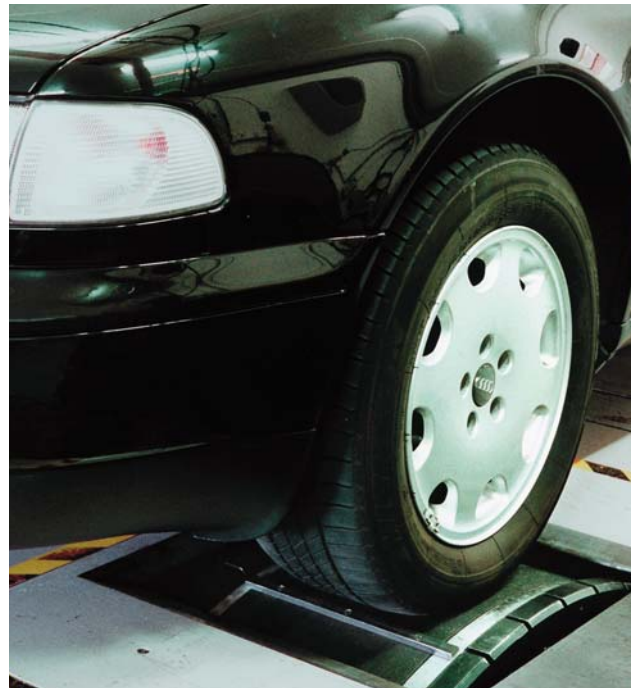
Rolling rig for mechanical and acoustic comfort tests
