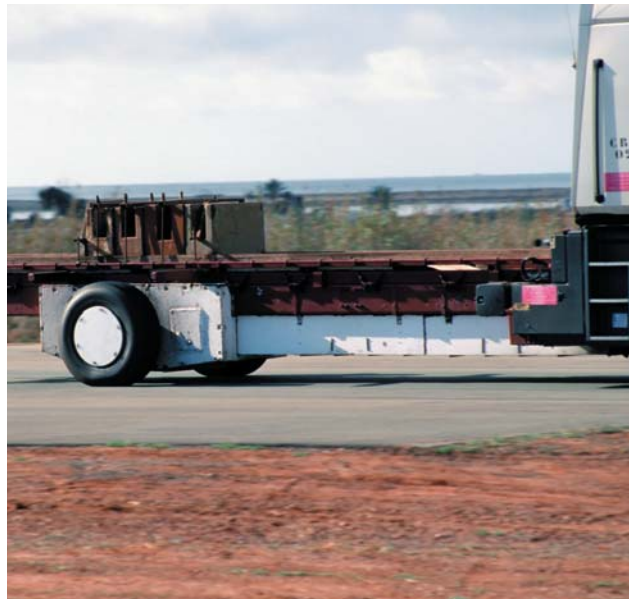
Truck whose transmission has been soundproofed with a foam-lined box.
