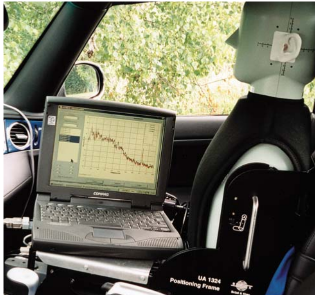
Dummy fitted with a microphone in each ear
