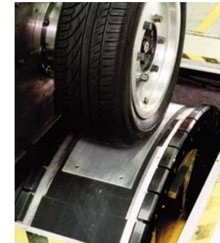
Drum for measuring loads at the wheel centre. Here the tyre is rolling over a plate 5 mm thick and 60 cm long.
