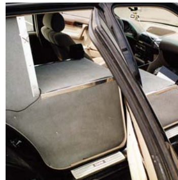
Here, the insulated exhaust system has been put inside the vehicle, in the place of the passenger's seat.
