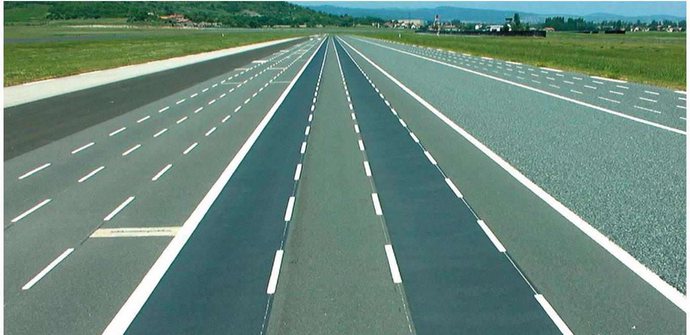
Test track with three types of road surface: macrorough, smooth, lane with isolated obstacles.
