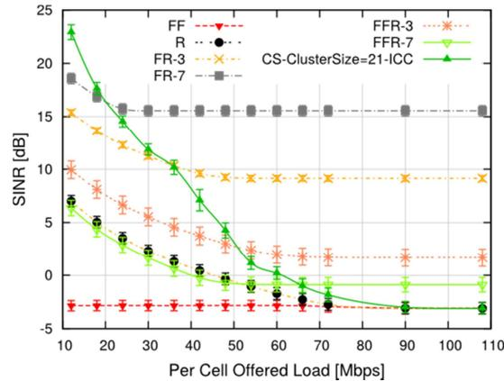
Figure 22 – 5th percentile of UEs' SINR, LTE-A scenario
