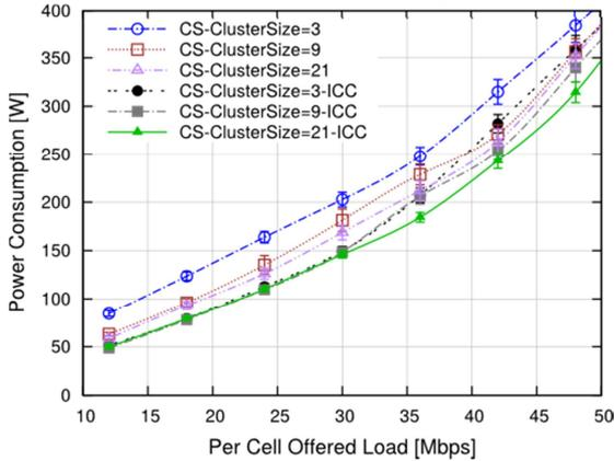
Figure 17 - Nodes' power consumption with different clustering
