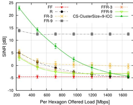
Figure 28 - 5<sup>th</sup> percentile of UE SINR, foreseen 5G scenario, micros enabled
