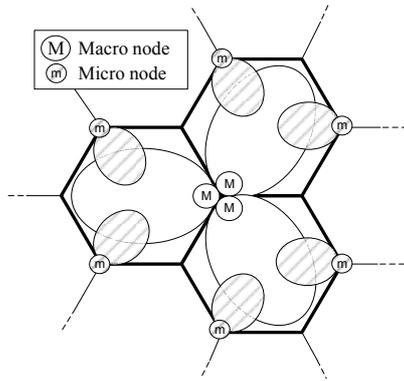
Figure 1 – Nodes in a hexagonal tessellation.
