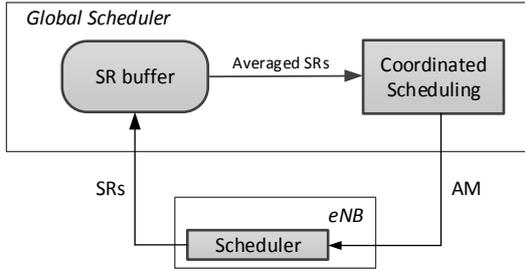
Figure 3 – Overview of Flex5Gware’s CS solution
