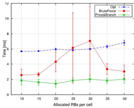
Figure 6 - Average solving times as a function of the cell load
