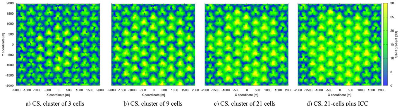
Figure 16 - SINR distribution, per-cell offered load=36Mbps
