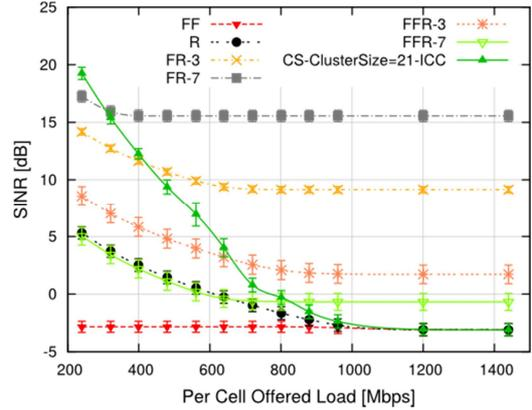
Figure 25 - 5th percentile of UEs' SINR, foreseen 5G scenario, macro-only than CS's. Note that 4G cells spend most of their time in very lightly loaded conditions, in practical deployments [31], hence schemes that allow a network to save energy when the load is low are going to make a remarkable difference in an operator's bill.
