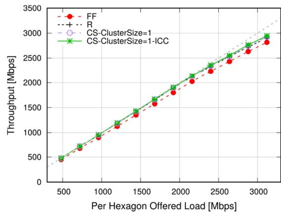
Figure 29 – Average per-hexagon throughput, dense deployment of pico nodes
