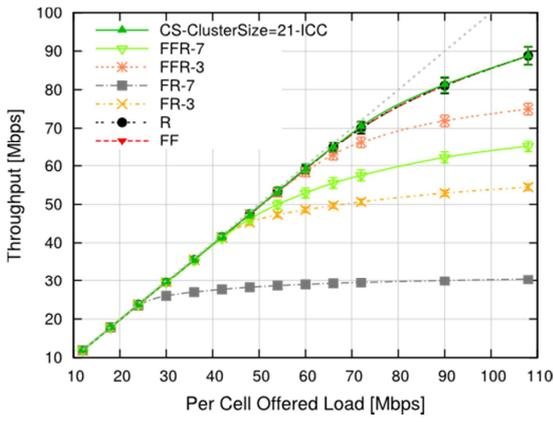
Figure 19 - Average cell throughput, LTE-A scenario
