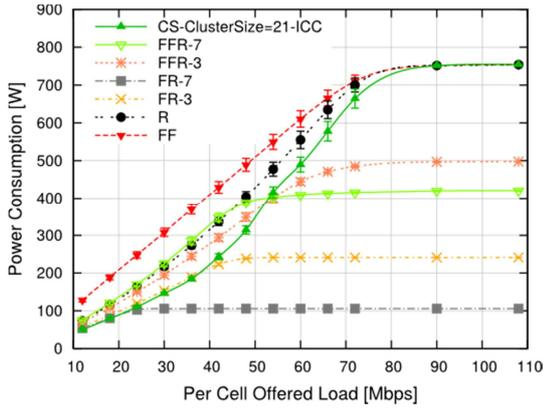
Figure 20 – Nodes' power consumption, LTE-A scenario
