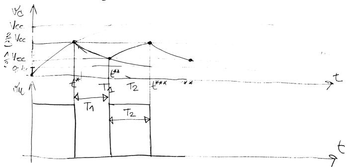
$$V_{c}(t) = (\frac{2}{3}V_{cc} - 0.2V_{cc})e + 0.2V_{cc}$$
