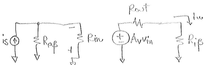
$$Ae = \left. \frac{i_u}{is} \right|_{\beta=0} = \frac{(R_{in} \parallel R_{of}) A_v}{R_{if} + Rout}$$
