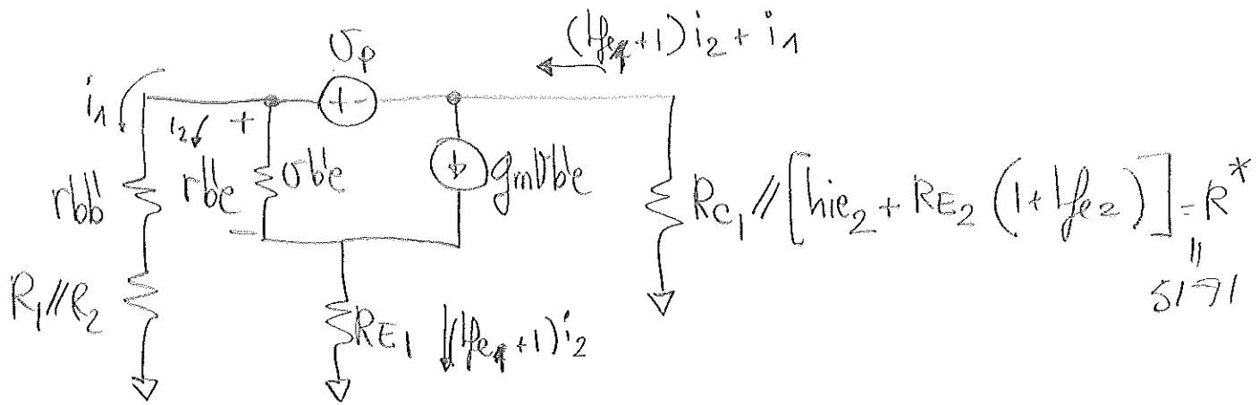
$$\therefore g_{mVbb} = g_m r_{bb}' i_2 = f_{fe1} i_2$$
