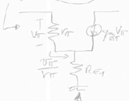
$$A_v = \frac{V_2}{V_1} = \frac{-\frac{q_m V_{TT} R_c}{R_{ff}}}{R_{ff} + R_{E1} \left( \frac{q_m V_{TT} + V_{ff}}{V_{ff}} \right)}$$
