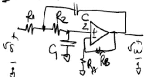
$$\frac{v_o}{v_i} = \frac{A_V}{R_1 R_2 C_1 C_2 s^2 + [(R_1 + R_2)C_2 + R_1 C_1(1-A_V)]s + 1}$$
