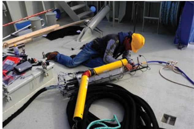
Figure 6. STU during a communication test on the Gunnerus deck before deployment. The two yellow cylinders are the KM modems, of which one is the STU's and the other is for testing. The gray box contains the STU electronics. Also visible in the photo is the blue cable used to connect the STU to shore, the black thermistor chain, and the hydrophone array.
