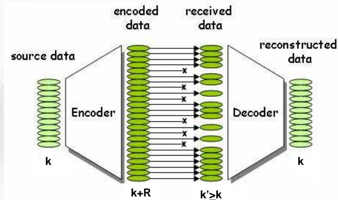
Any subset of  $k$  encoded blocks allows the receiver to reconstruct the source data
