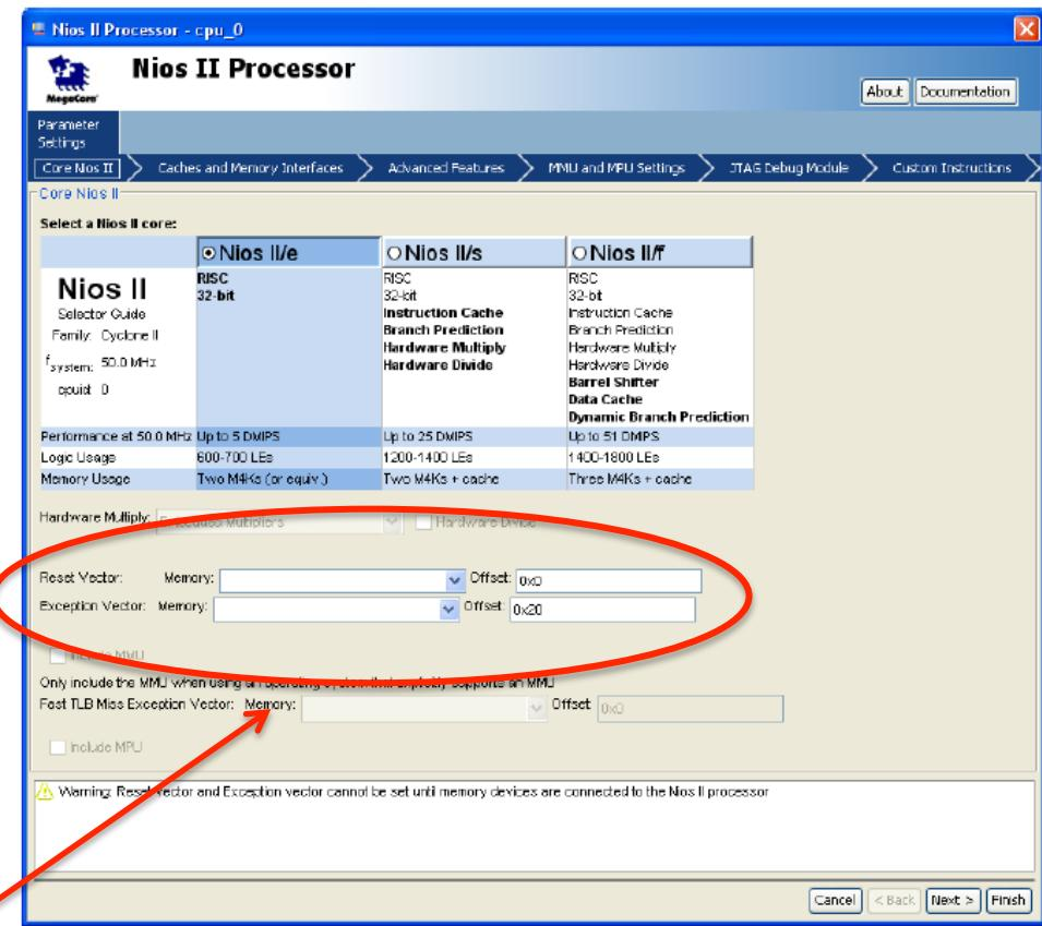
At least one memory must be present in the Qsys system in order to configure the **Reset** and **Exception** addresses
