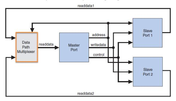
In Qsys the generation of data path multiplexing logic is specified using the Connections column on the System Contents tab
