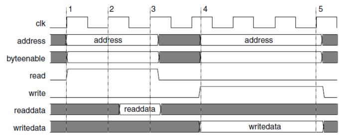
Pipelined w/ waitrequest and fixed wait states (readWaitTime =2) . Signals at the slave interface
