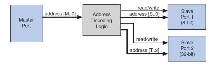
The address decoding logic is controlled by the Base address setting in Qsys
