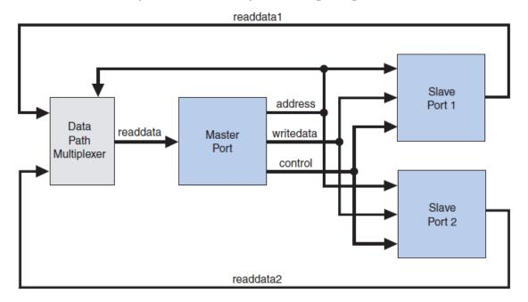
• In **Qsys** the generation of data path multiplexing logic is specified using the connections panel on the System Contents menu
