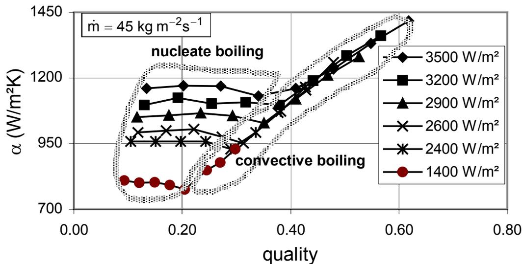
Figure 8 A graph of heat transfer coefficient against heat flux showing nucleate boiling and convective heat transfer regions, Feldman et al [27]
