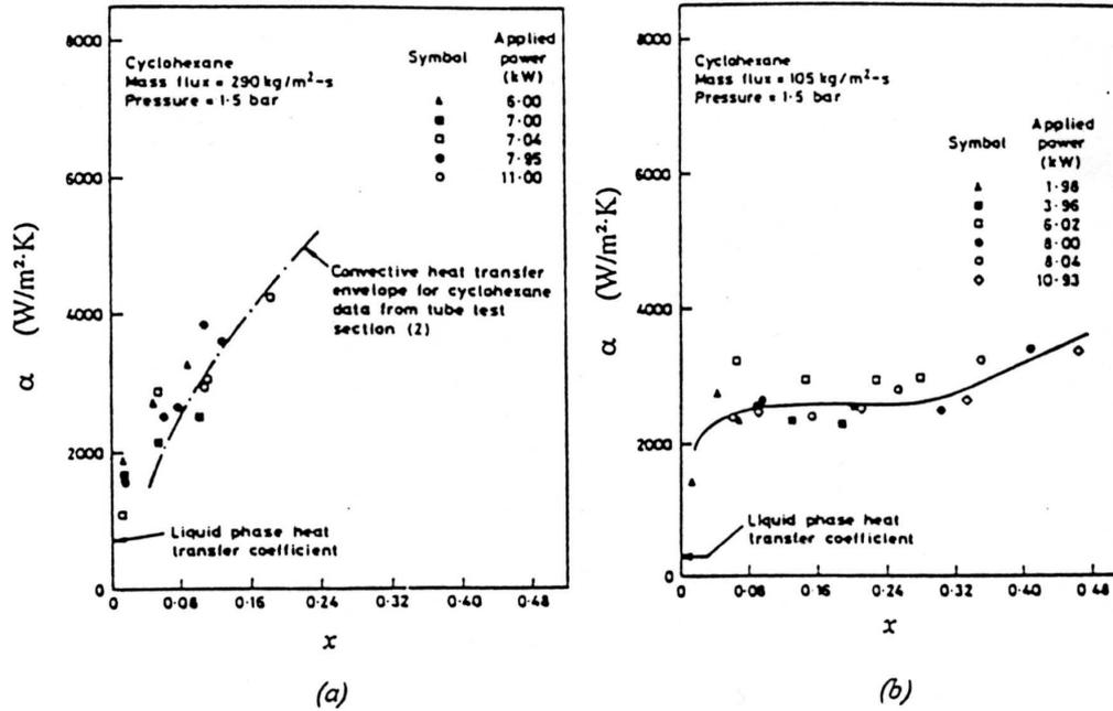
Figure 7 Plot of boiling heat transfer coefficient against quality for two different mass flux values, Robertson and Wadekar [23].
