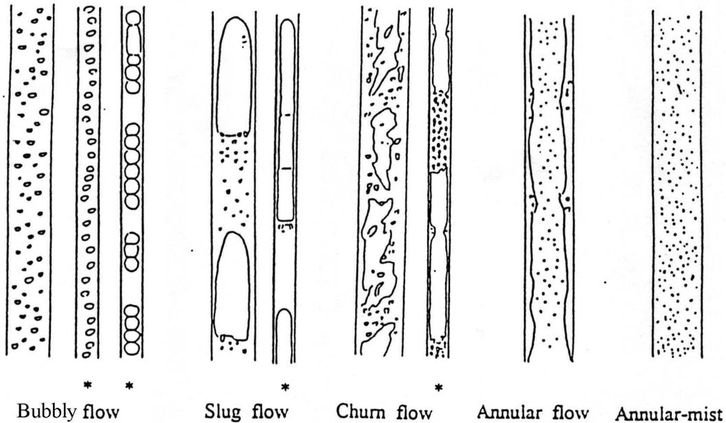
Figure 11 Effect of tube diameter on flow patterns, from Mishima and Hibiki [39]
