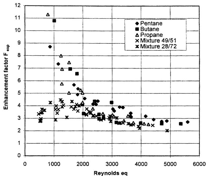
Figure 10: Condensation in a cross-corrugated compact heat exchanger by Gitteau et al [35]
