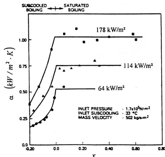
Figure 1 Local heat transfer coefficient as a function of local vapour quality for 3.1 mm diameter tube at different heat flux values, Lazarek and Black [7].
