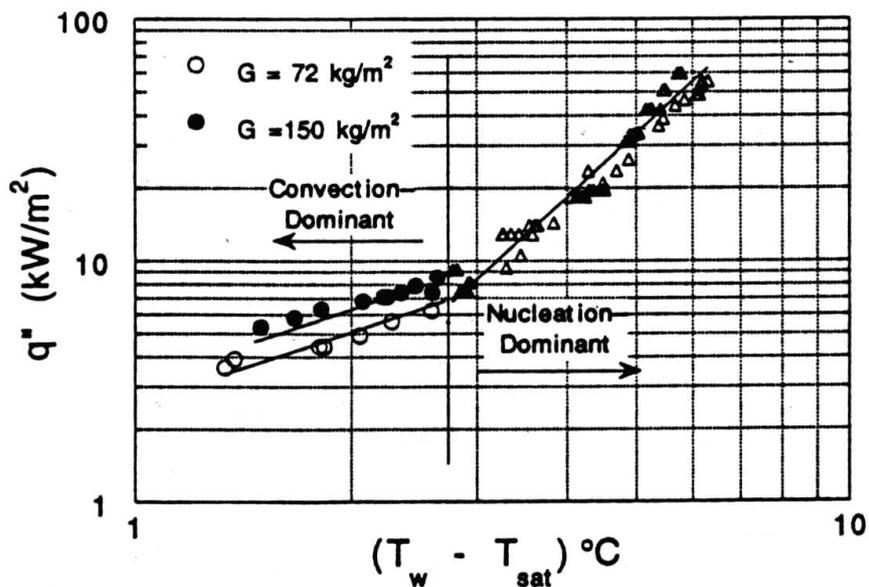
Figure 2 A graph of heat flux against wall superheat showing nucleate boiling and convective heat transfer dominated regions, Tran et al. [9].
