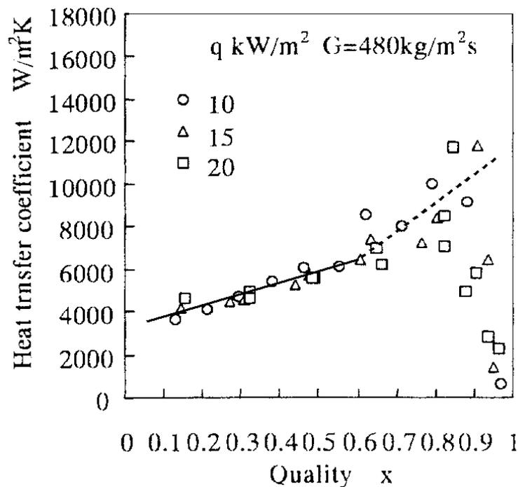
Figure 5 Measured data of Oh et al [12] for flow boiling of R134a in a 2 mm diameter tube. Best fit lines show two regions of convective heat transfer.
