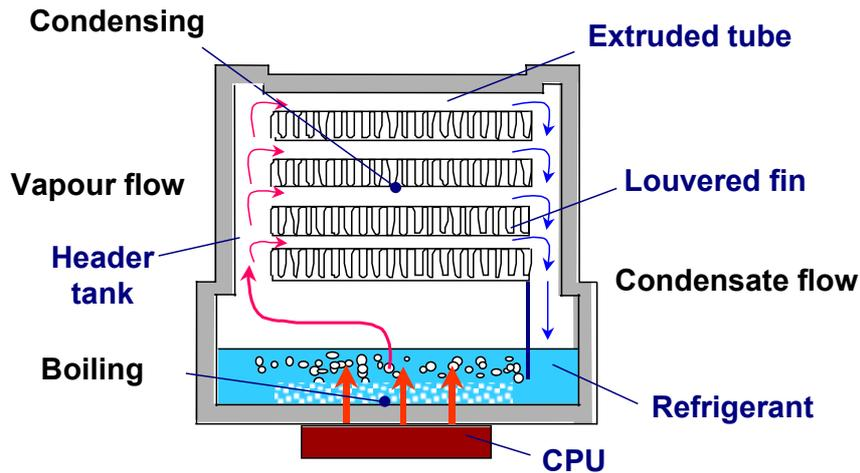
Figure 17 A novel plate-fin design for high heat flux of cooling of electronic devices [52]
