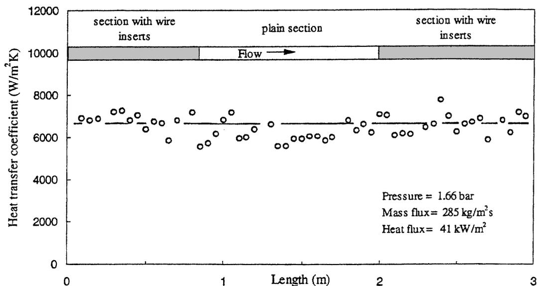
Figure 14 Typical flow boiling results from a composite test-section with wire inserts [45]
