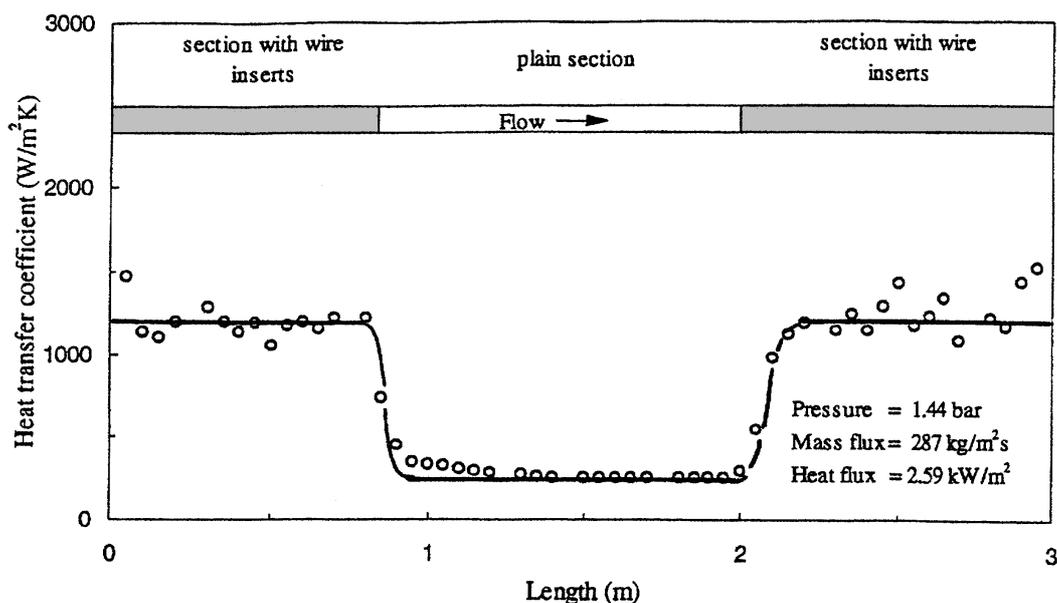
Figure 13 Typical single phase results from a composite test-section with wire inserts [45]
