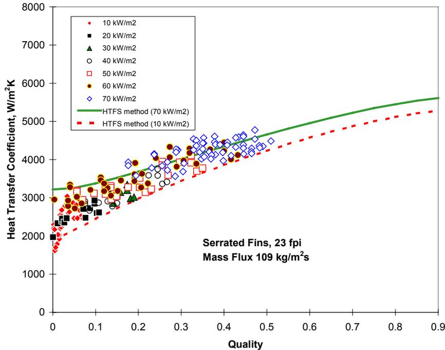
Figure 15 Predictions of the HTFS method and recent HTFS data for flow boiling of pentane
