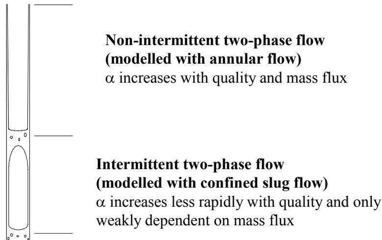
Figure 12 Schematic diagram showing two main flow patterns for small diameter tube and parametric trends in absence of nucleate boiling
