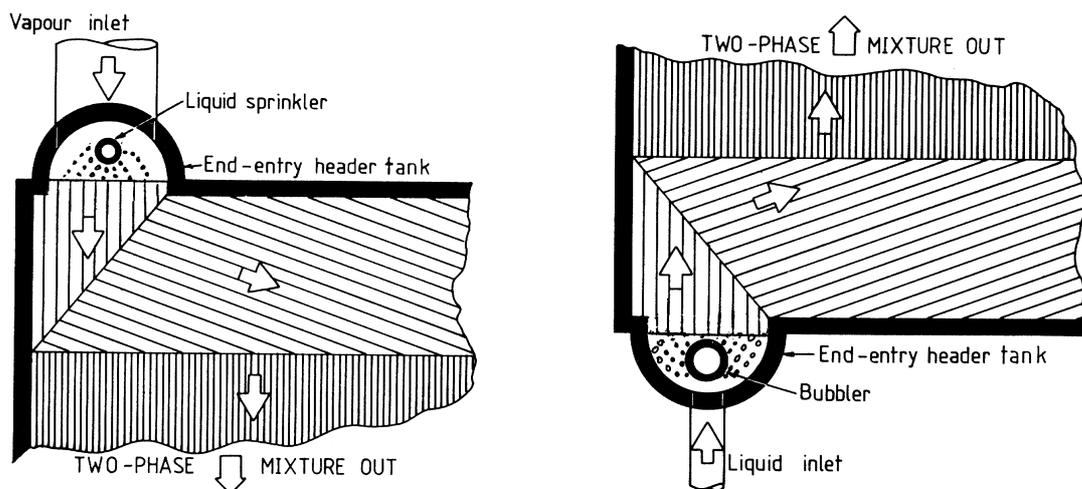
Figure 16 Spray remixer and bubbler remixer for distributing the phase in the exchanger header tank [47]
