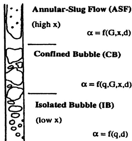
Figure 6 Flow regimes in a narrow diameter tube, Cornwell, Kew and co-workers [14,15]
