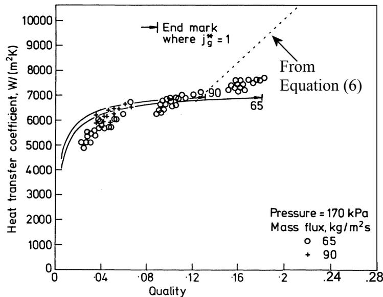
Figure 12 Two distinct regions of different trends of two-phase convective flow boiling heat transfer, adapted from Wadekar and Kenning [37]
