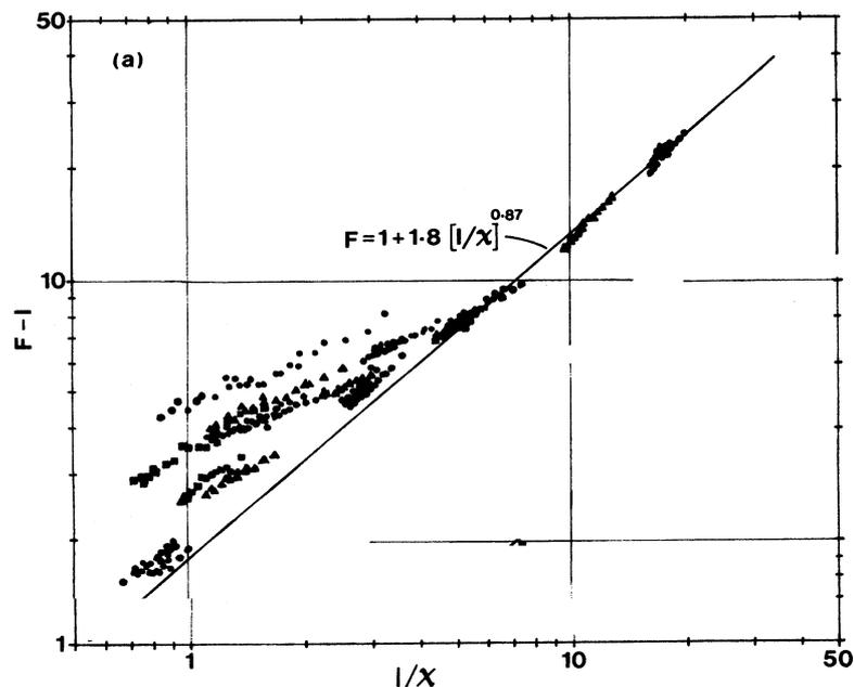
Figure 11 Data for flow boiling of water in a 14.4 mm diameter tube, Kenning and Cooper [36]
