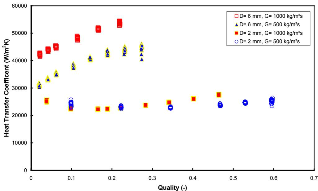
Figure 4 Local heat transfer coefficient as a function of vapour quality using the data in saturated flow boiling, adapted from Kureta et al [11]
