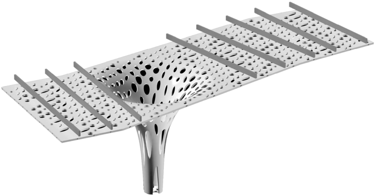
Main canopy and funnel: rendered view with GRP cladding
