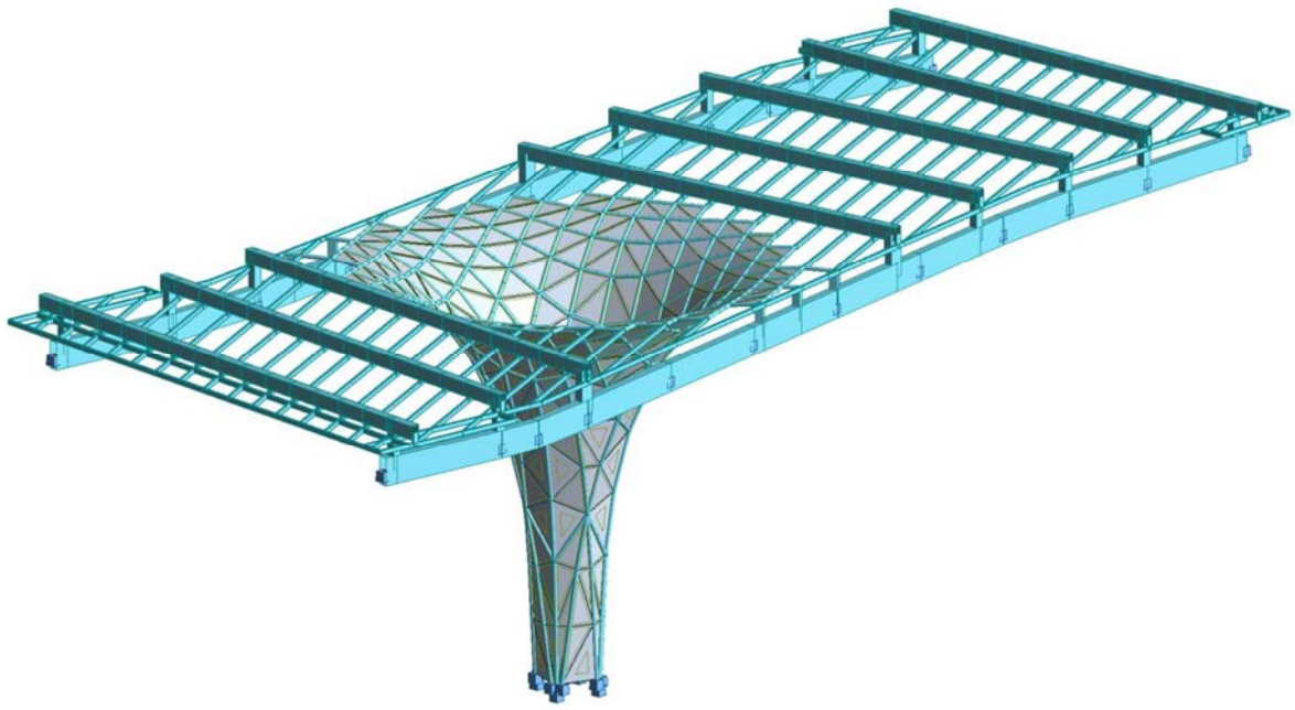
Main canopy and funnel: structural model in Robot
