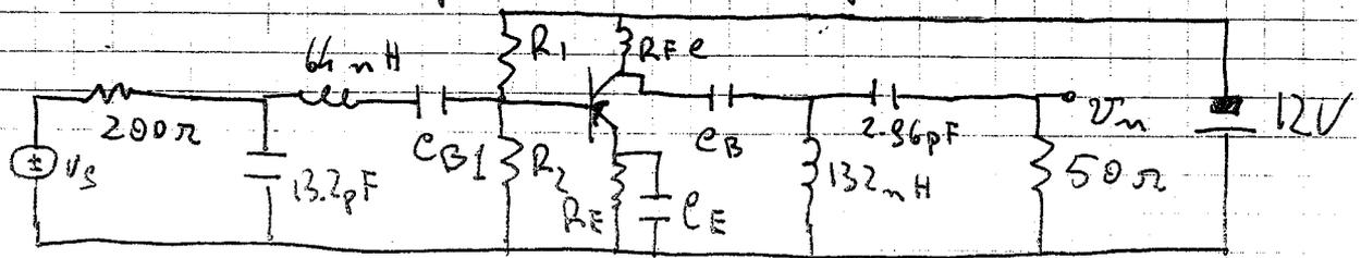
$$R_E = 1 \text{ k}\Omega \quad V_B = -2.7 \text{ V} \quad R_2 = 13.5 \text{ k}\Omega \quad R_1 = 46.5 \text{ k}\Omega$$
