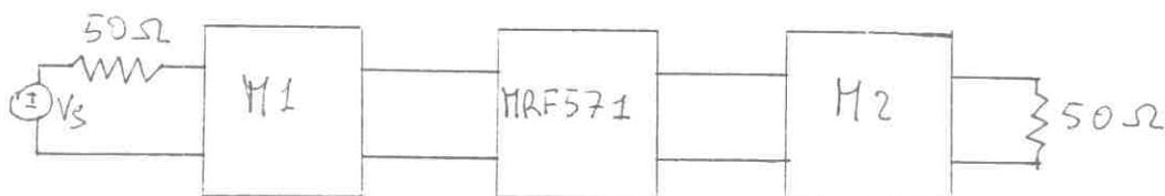
$$V_s = v_{sn} \cos \omega_0 t; \quad \omega_0 = 2\pi f_0; \quad f_0 = 500 \text{ MHz}; \quad v_{sn} = 0.1 \text{ V.}$$
