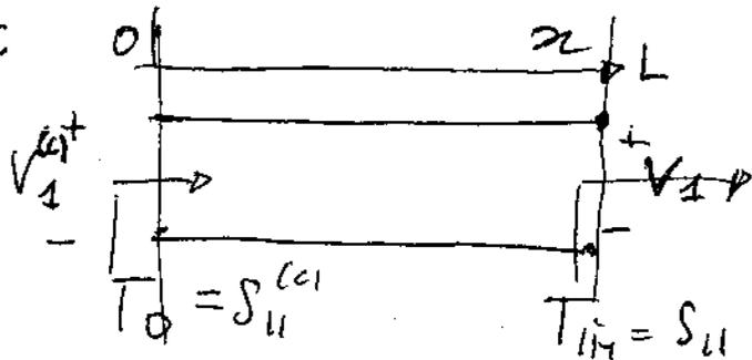
$$V_1^{(cc)} = V^+ + V^- = V^+ (1 + \Gamma_0)$$
