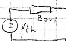
$$P_{\text{OUT}} = P_{\text{BL}} = 82 \text{ mW} = \frac{V_{TH}^2}{8 \cdot R_{\text{OUT}}} \Rightarrow V_{TH} = 2.3 \text{ V}$$
