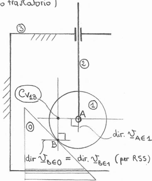
5)  $\underline{a}_{AE1} = \underline{a}_{BE1} + \ddot{\theta}_1 \underline{k} \times \underline{BA} - \dot{\theta}_1^2 \underline{BA} = r \dot{\theta}_1^2 \underline{n} + \ddot{\theta}_1 \underline{k} \times \underline{BA} - \dot{\theta}_1^2 \underline{BA}$ , con  $\underline{n} = \frac{\underline{BA}}{\|\underline{BA}\|} \equiv (\frac{\sqrt{2}}{2}, \frac{\sqrt{2}}{2}, 0)$
