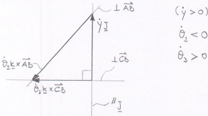
3)  $\dot{y} \underline{j} + \begin{vmatrix} \underline{i} & \underline{j} & \underline{k} \\ 0 & 0 & \dot{\theta}_2 \\ AB_x & AB_y & 0 \end{vmatrix} = \begin{vmatrix} \underline{i} & \underline{j} & \underline{k} \\ 0 & 0 & \dot{\theta}_3 \\ 0 & d & 0 \end{vmatrix}$ , con  $\begin{cases} AB_x = b+e \\ AB_y = -(b+e) \tan 30^\circ = -\frac{b+e}{\sqrt{3}} \end{cases}$
